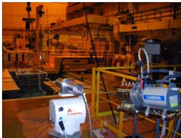
Fig. 9: Gamma Camera and In Situ Spectrometer System (ISOCS) Gamma probe positioned in UP1 plant
