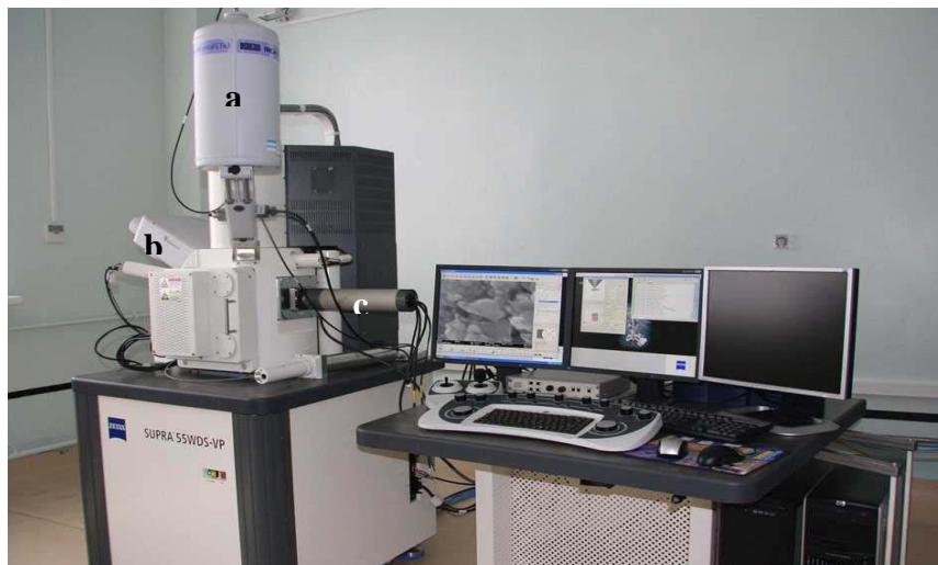
Fig.1. Super-high resolution field-emission scanning electron microscope Zeiss SUPRA55VP, Carl Zeiss AG, Germany, energy-dispersive spectrometer Inca Energy 350 (a), wave spectrometer Inca Wave 500 (b) and HKL EBSD Premium system for registration and analysis of backscatter electron diffraction. (c).
