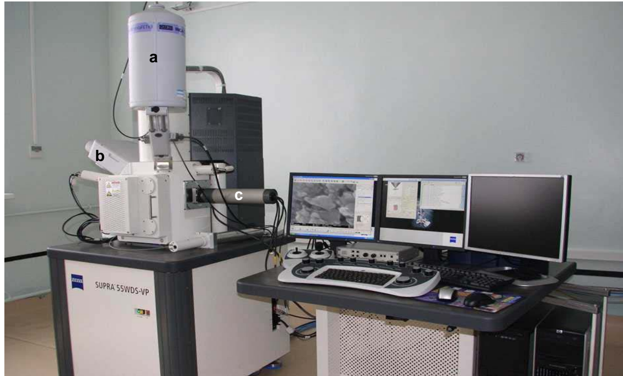
Super-high resolution field-emission scanning electron microscope Zeiss SUPRA55VP, Carl Zeiss AG, Germany, energy-dispersive spectrometer Inca Energy 350 (a), wave-dispersive spectrometer Inca Wave 500 (b) and HKL EBSD Premium system for registration and analysis of backscatter electron diffraction. (c).
