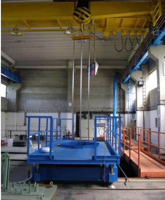
Fig. 8. Platform for loading of SNF from the pool.
