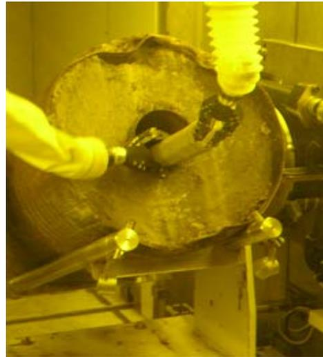
*Fig. 4. Removing of FA from the storage drum.*
