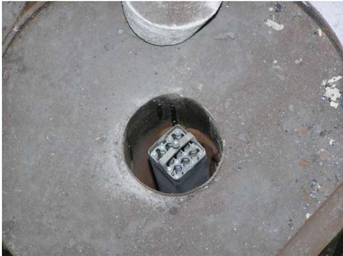
*Fig. 3. View inside one EK-10 storage drum after plug removal.*
