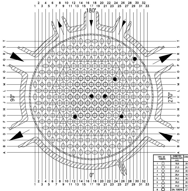
FIG. 3.2. Plan view of reactor lattice, the position pointed in black are the CC under follow-up.
