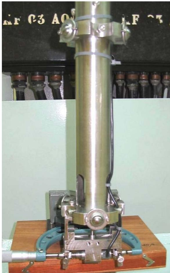
*FIG. 3.6. Self centered ID gauging head, during calibration.*
