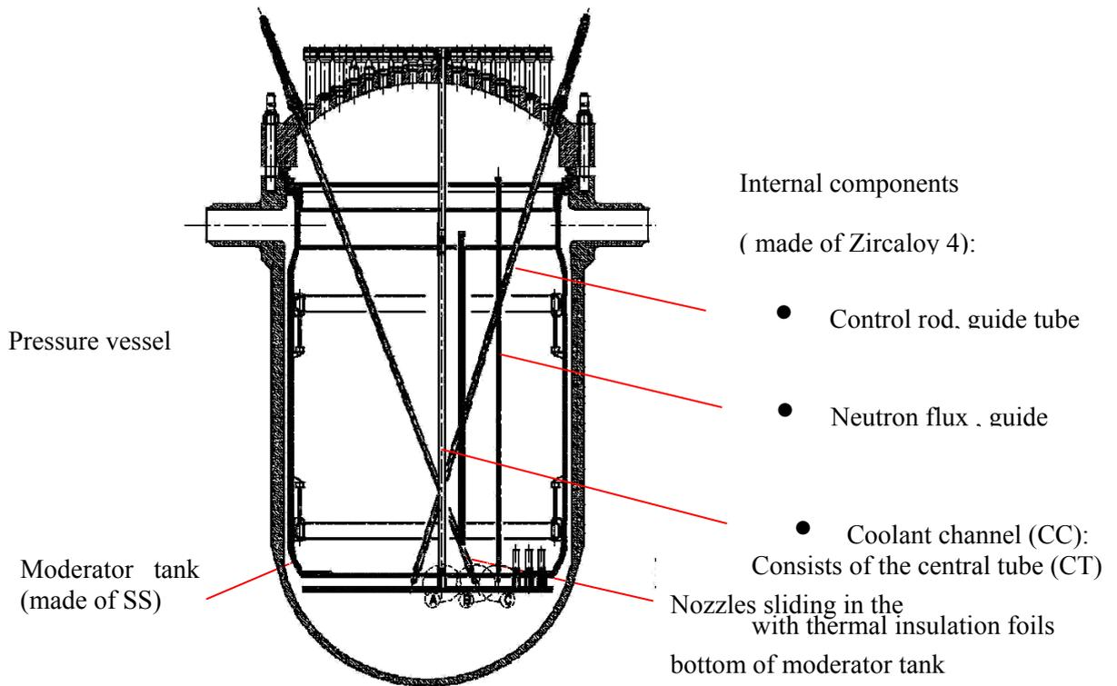
FIG. 2.1. Simplified cut view of Atucha-1 reactor.
