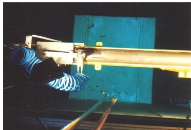
FIG. 3.9. A pneumatic motor driven by a trolley and sliding over the grey is cutting and extracting the sample of CT and insulation foil.
