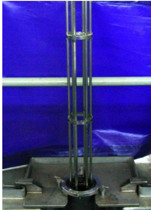
FIG. 3.4. Shows the ruler during the introduction in the CC for the length measurement.
