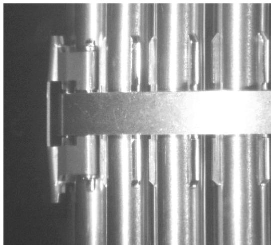
FIG. 3.13. Evaluation of relaxation and wearing from the visual inspection of the side view of elastic shoes.
