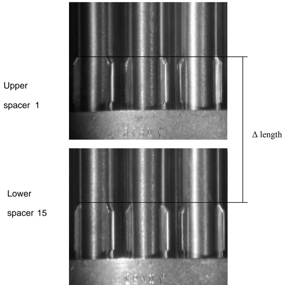
FIG. 3.1.4. Reference level taken at the rigid pads (central rod) from an image of the periscope to measure the rod length. Resolution 0.5 mm.
