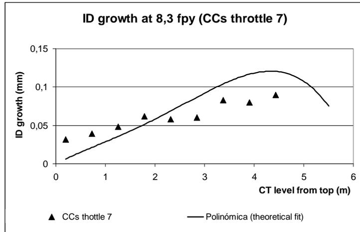
FIG. 3.7. Comparison of measured ID growth with the theoretical profile predicted by code calculation. (Values are the average of two CCs with throttle 7, maximum dose).
