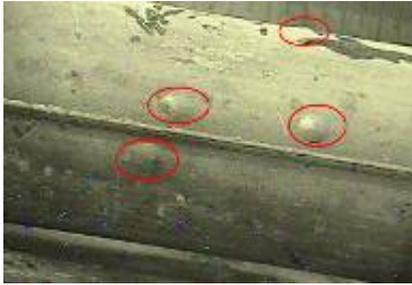
FIG. 3.9. 12 Blistering of fuel tube.
