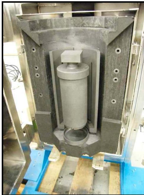
*FIG. 5.2 Retort (sample holder) mounted inside main furnace.*
