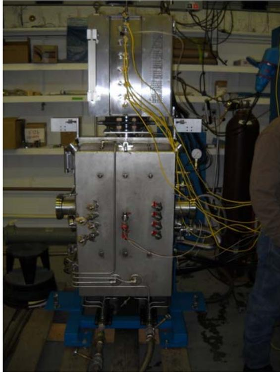
*FIG. 5.1. Main furnace and thermal gradient furnace at the bottom and top respectively.*
