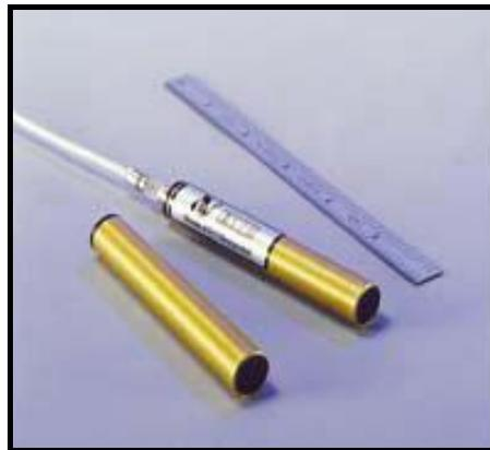
FIG. 5.5 Example SPEAR detectors.
