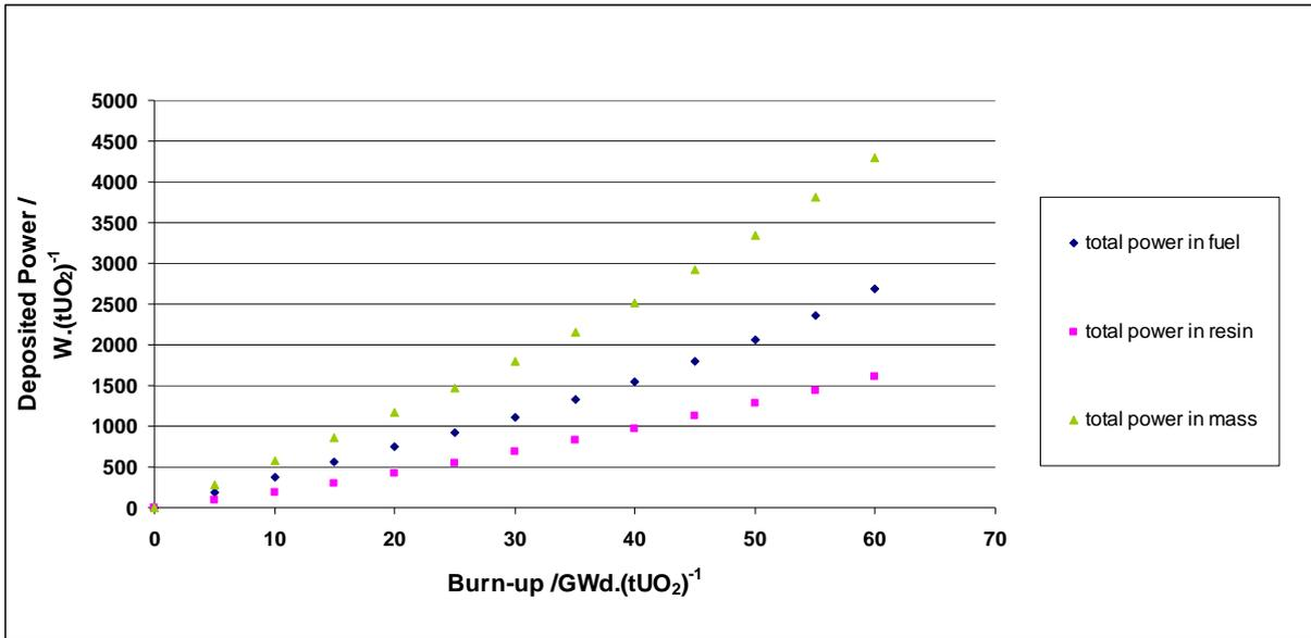
FIG. 5.1. Total power deposition in resin and fuel with burn-up after a 5 year cooling time.
