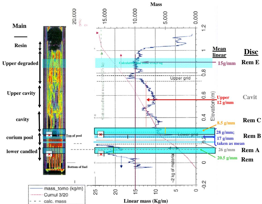
FIG. 2.3. Diagram giving the linear masses of the various remnants of the FPT1 bundle that have been selected for analysis of H<sub>2</sub> gas evolution along with their position in the bundle.
