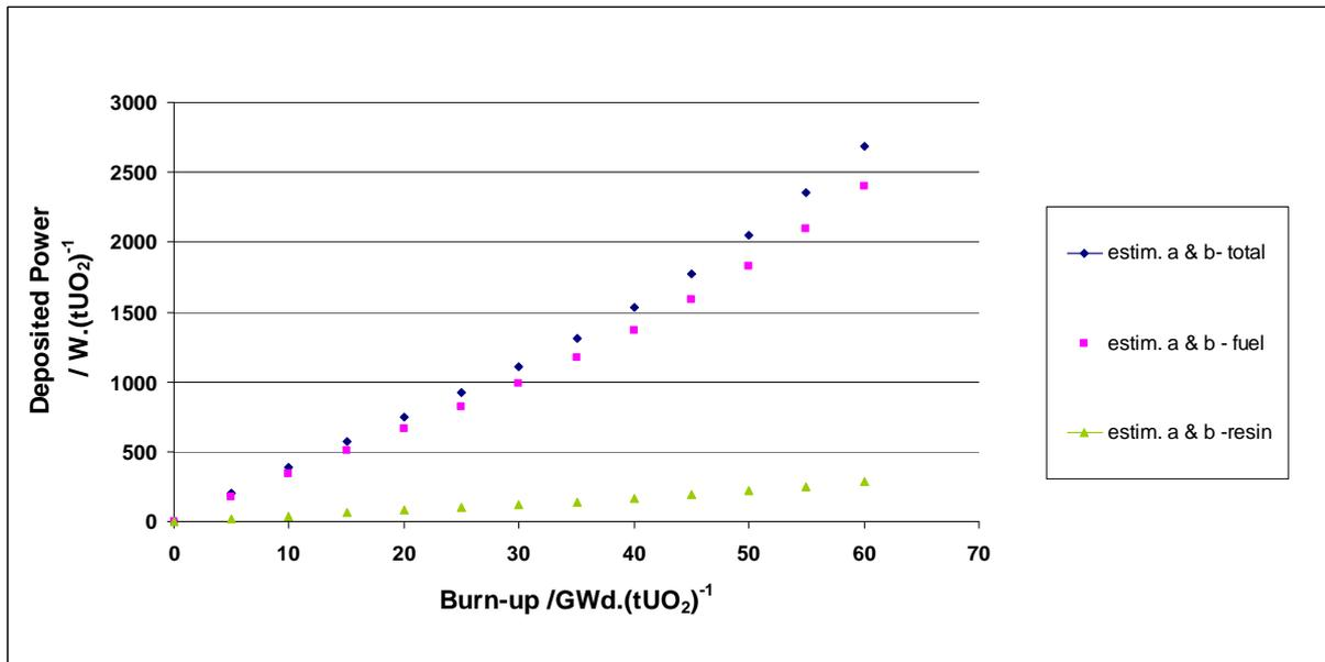
FIG. 5.4. Alpha and beta power deposition in resin and fuel with burn-up after a 5 year cooling time.
