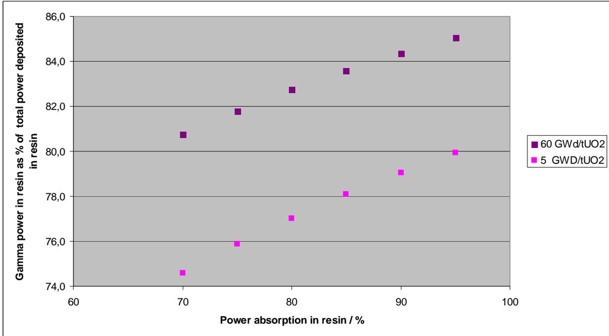
FIG. 5.5 Variation of gamma power deposited in resin as a percentage of total deposited power in resin with division of gamma power deposition from 30% fuel -70% resin to 5 % fuel and 95% resin for a high and low burn-up fuel after a 5 year cooling time.
