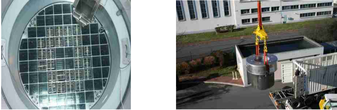
FIG. 4.1. 26 U-Al spent fuel assemblies from Osiris MTR have been placed inside the TN-MTR cask (left), and shipped from Saclay (right) to La Hague.
