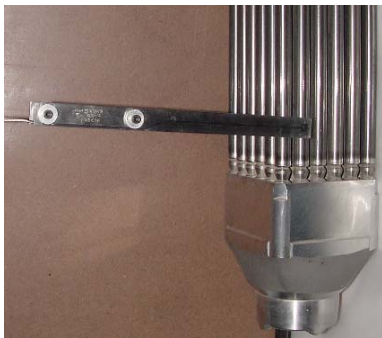
FIG. 5.1. 100% signal for sound fuel rod.
