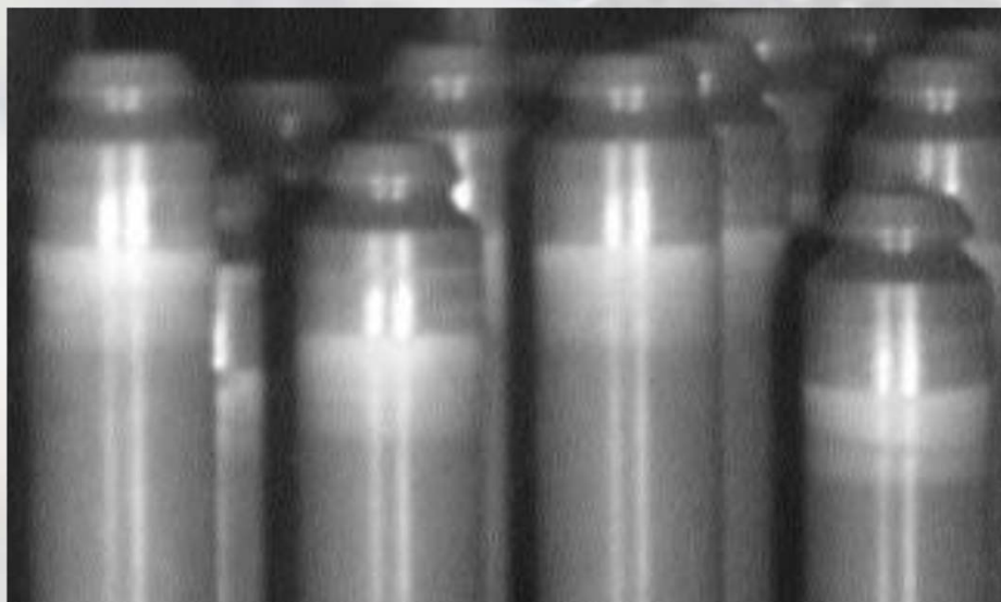
Weld Joints of Top End Plugs after 4 cycles
