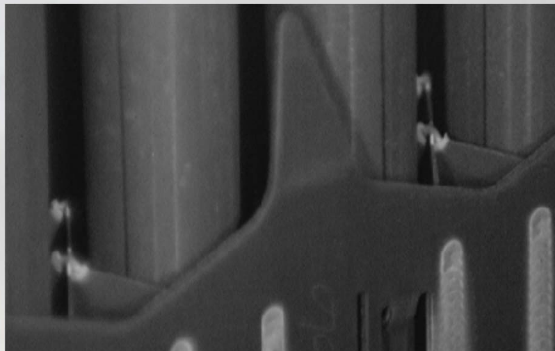
Zr1%Nb Grid 14 Weld Joints after 2 cycles
