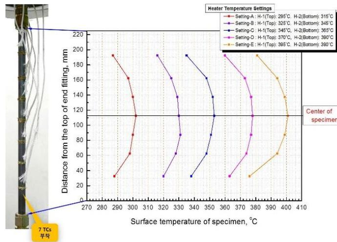
Figure 5. Axial temperature distribution along the cladding specimen
