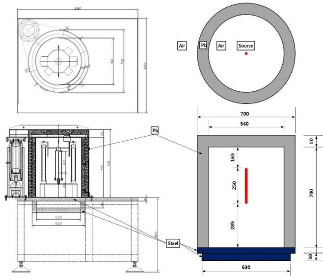
Figure 2. Geometrical modeling for radiation shielding analysis of fatigue test machine
