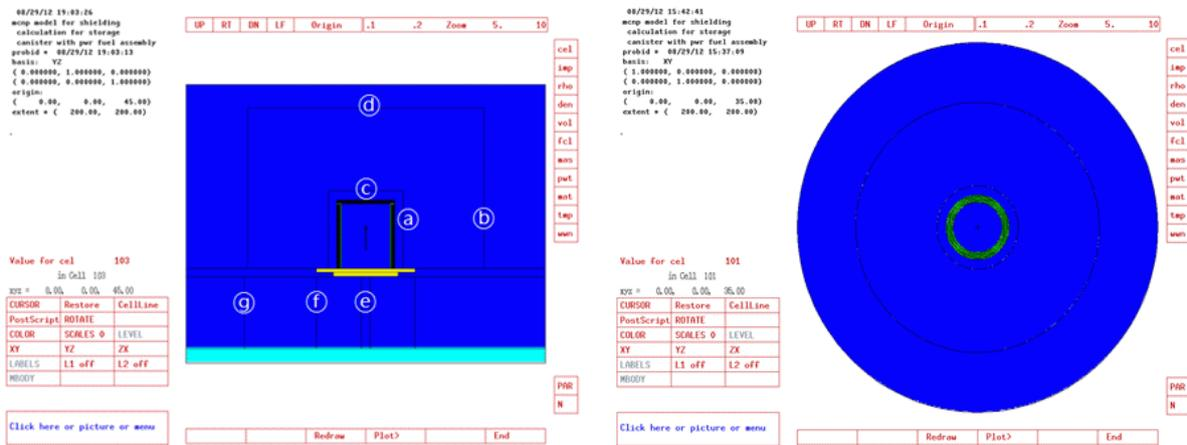
Figure 3. MCNP model for radiation shielding calculation
