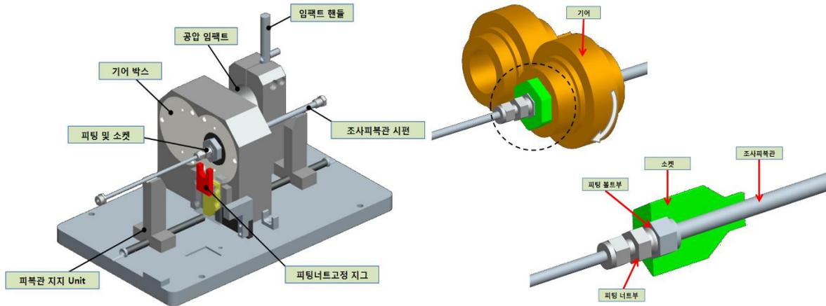
Figure 4. Schematic diagram of fitting fastening apparatus in hot cell
