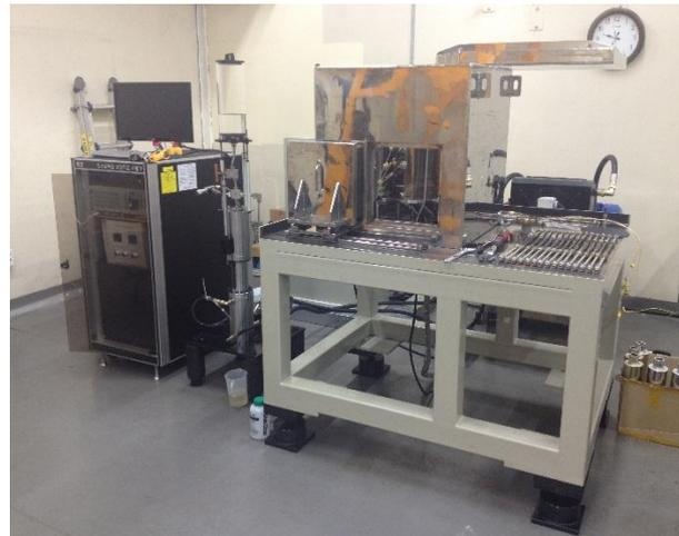
Figure 1. Schematic diagram and image of cyclic pressurization fatigue tester
