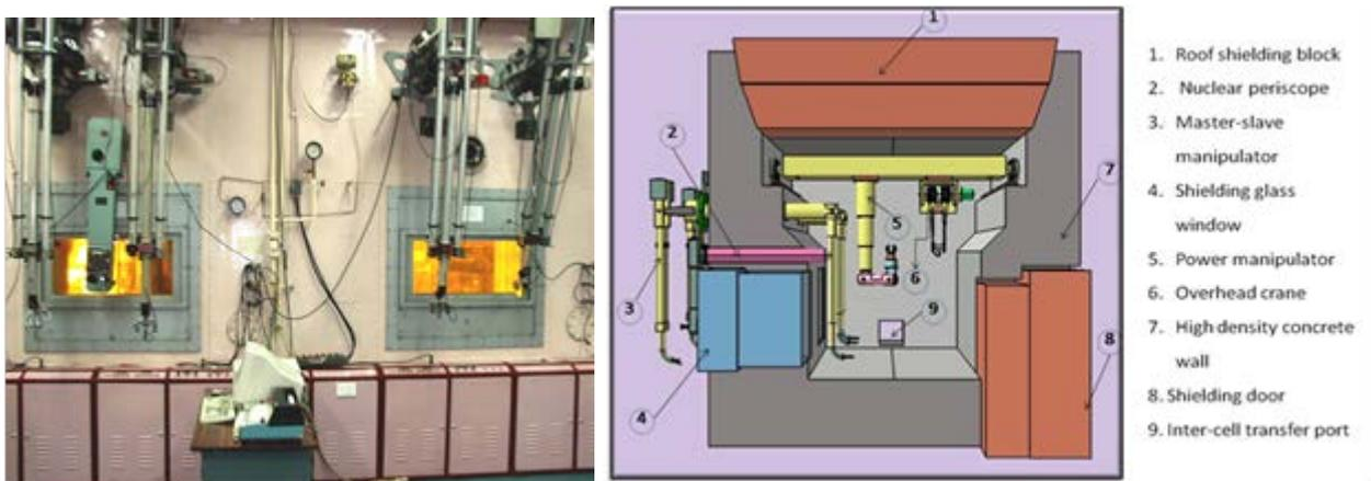
Fig 1 a. Front view of an RML hot cell Fig 1 b. Typical cross sectional view of a Hot cell
