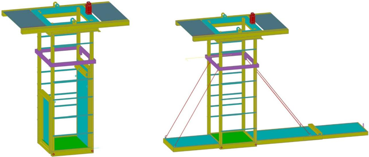
Fig 6 Sketch of the Man Entry System (MES I): folded and unfolded states.
