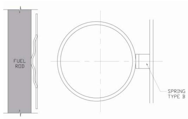
Fig. 4. Shape of the cell spring.
