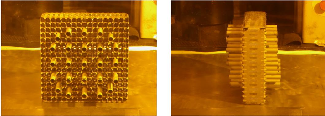
Fig. 2. Irradiated spacer grid obtained for the measurement of spring stiffness and dimensional change in a hot cell.
