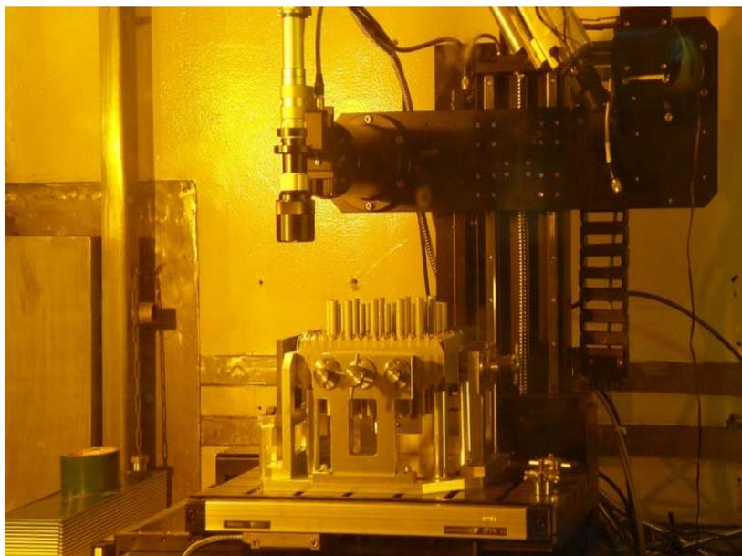
Fig. 7. Experimental set-up for the measurement of the grid in a hot cell.
