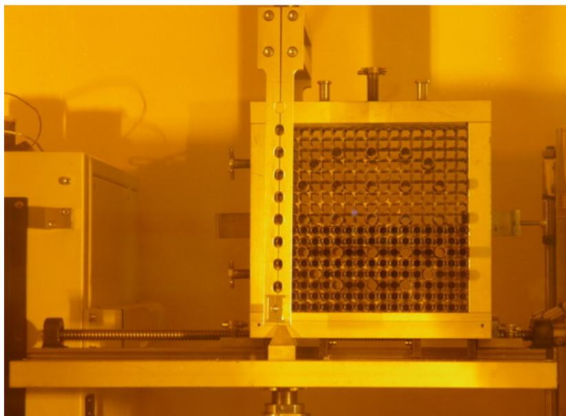
Fig. 5. Grid cell spring test in a hot cell.
