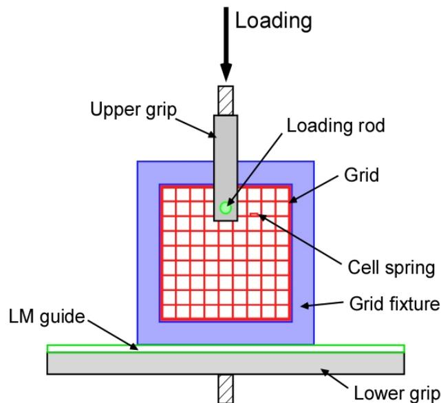
Fig. 3. Schematic diagram of grid cell spring test.
