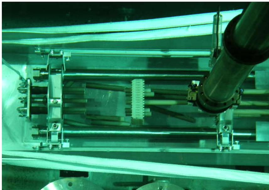
Fig. 1. Cutting machine to cut the guide thimbles and instrumentation tubes simultaneously at both sides of a grid using abrasive wheels.
