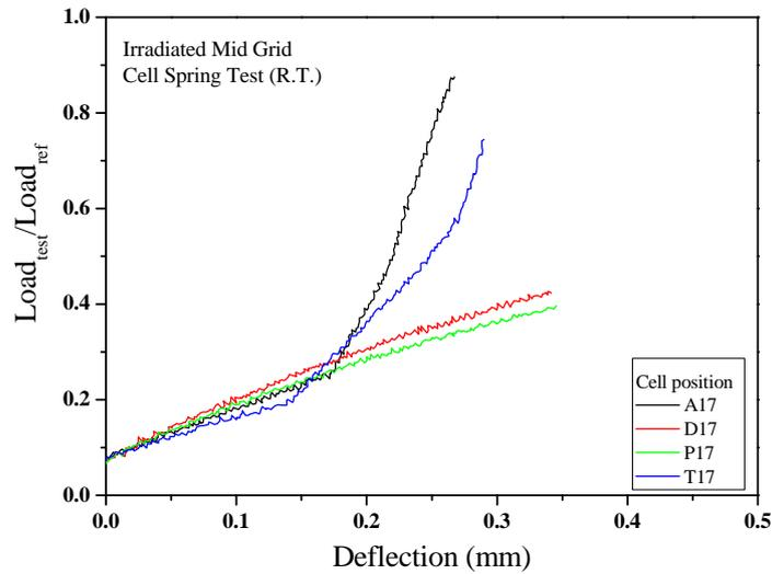
Fig. 6. Load-deflection curves of grid cell spring tests.
