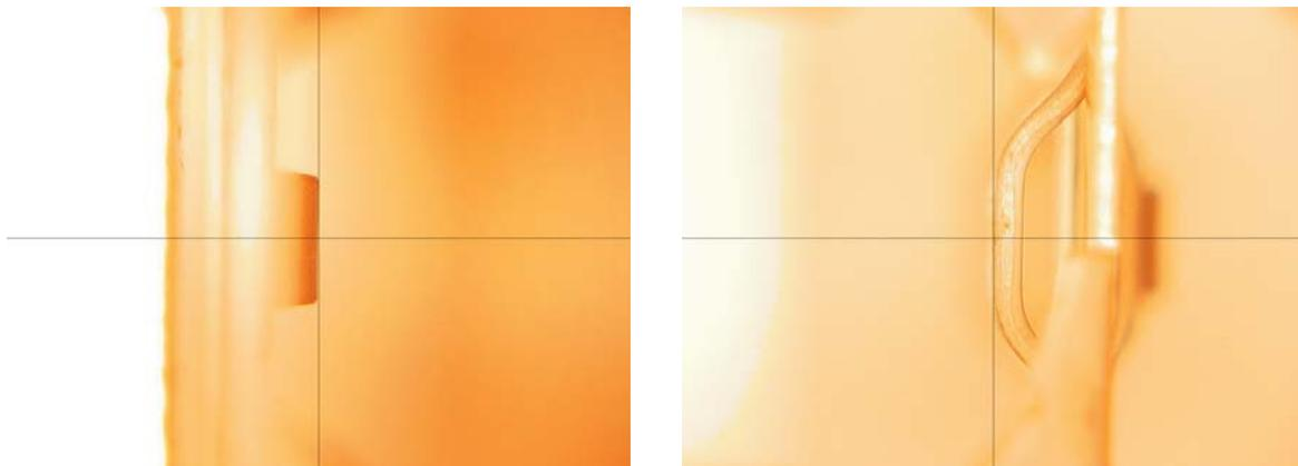
Fig. 8. Spring and dimple images obtained from a CCD camera for the dimensional measurement
