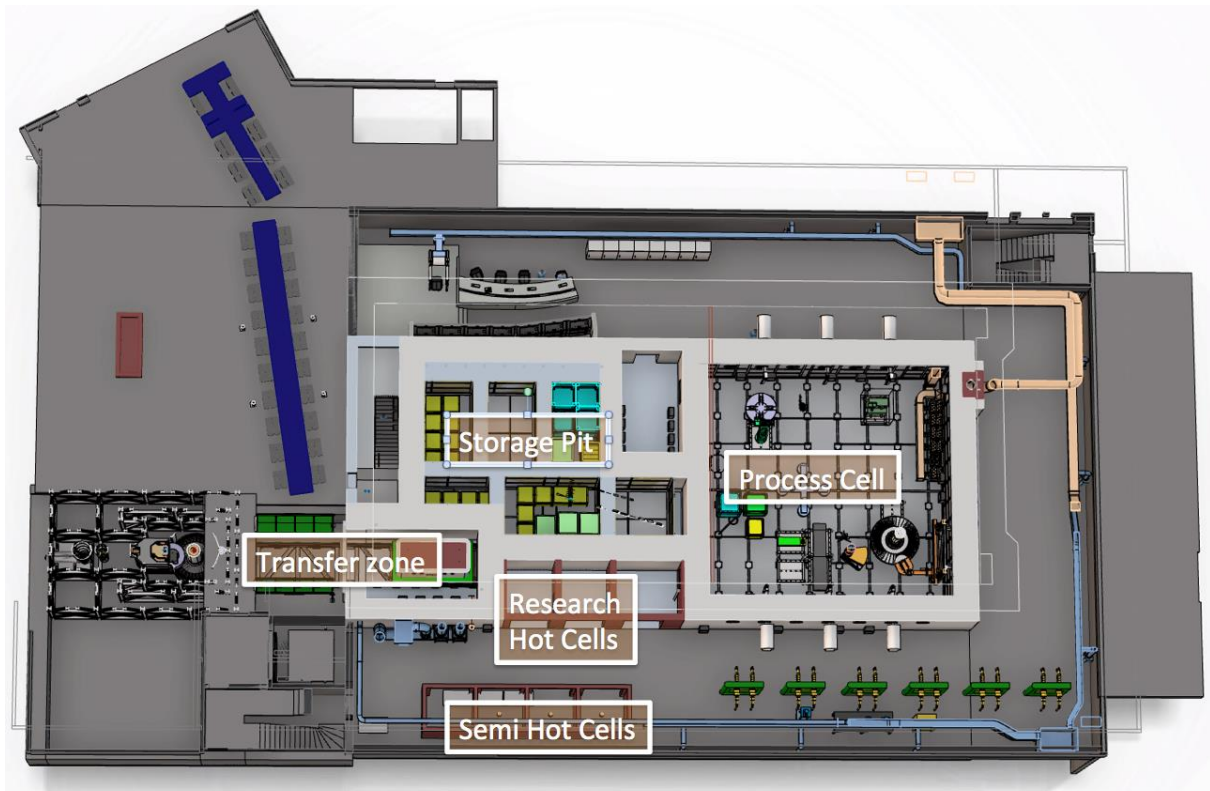
Figure 5: Top view of research hot cells and its integration to the active cell system, where three subsystems, the process cell, the storage pits and the transfer zone of the active cell system are shown.
