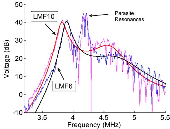
Fig. 5. Experimental response of LMF6 sensor (black curve) and LMF10 sensor (red curve).
