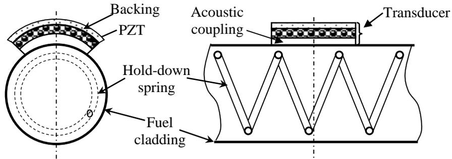
Figure 1. Schematic representation of measurement process, tube inner diameter  $D=8.36$  mm and tube thickness  $e=0.57$  mm (from [1]).
