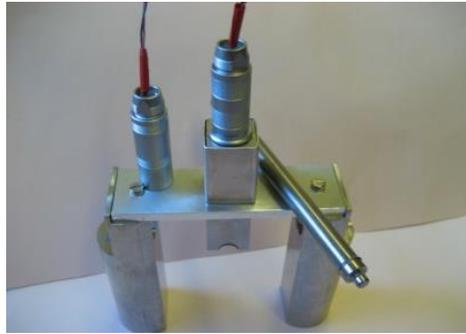
Fig. 2. A specific acoustic sensor for hot cell measurements including auto-positioning system and LEMO connector from [6].
