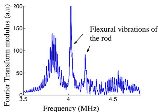
Fig. 3. Spectral response of the system between 3.5 and 5 MHz. The sharp peaks correspond to the gas resonance. The two flexural vibrations of the rod are the main parasites.
