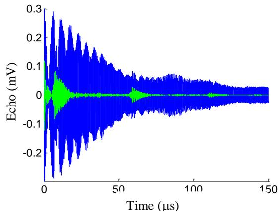
Fig. 4b. Time domain response in the case of the signal is low (blue curve). The echoes are in the noise. After a signal treatment, parasites are separated and gas echoes appear (green curve).
