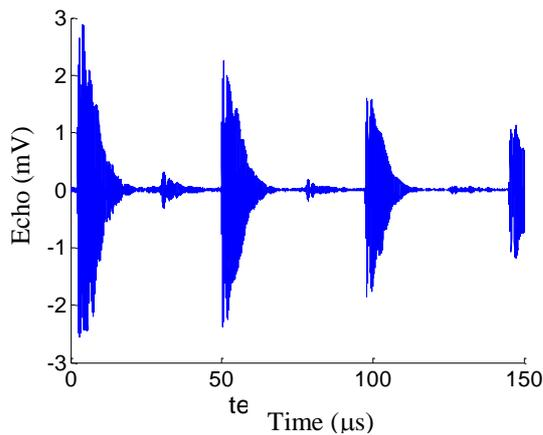
Fig. 4a. Time domain response for a rod without a spring and for 150 bars pressurised gas. The resonances of the gas have a high amplitude which constitutes the major part the signal. The echoes are separated from noise.
