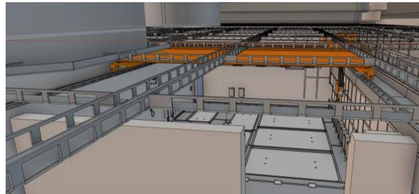
Fig 4. Example of in-concrete liner beams
