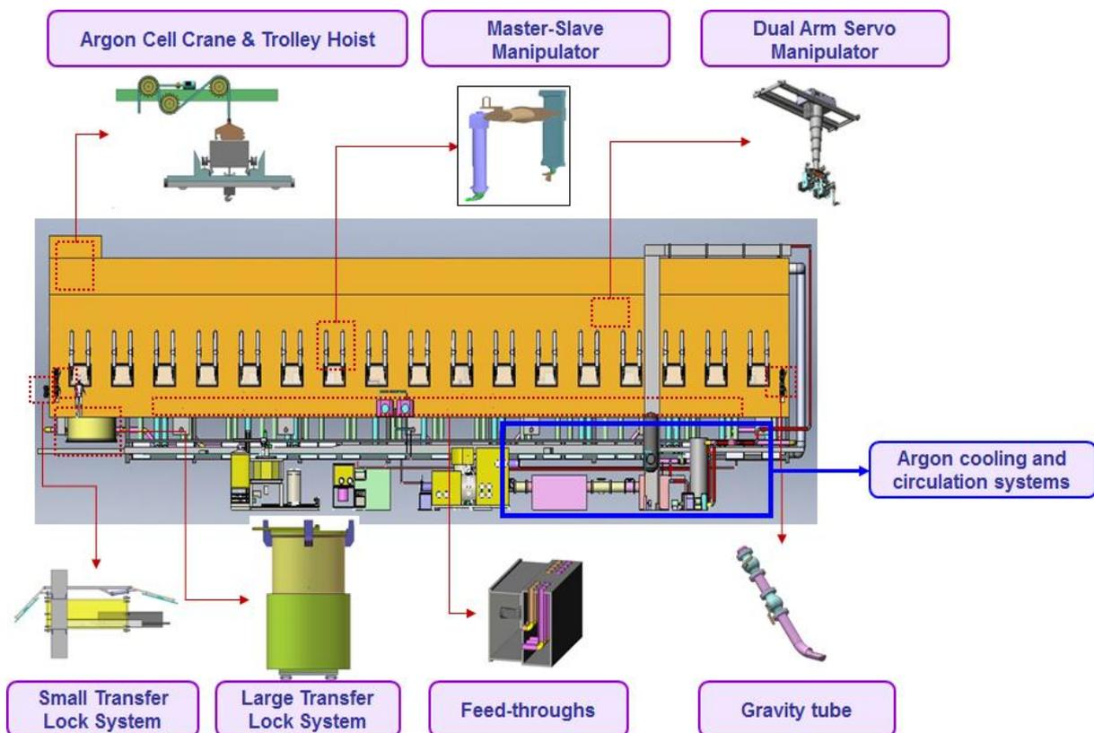
Figure 2. Isometric section view of PRIDE with cell equipment and remote handling systems
