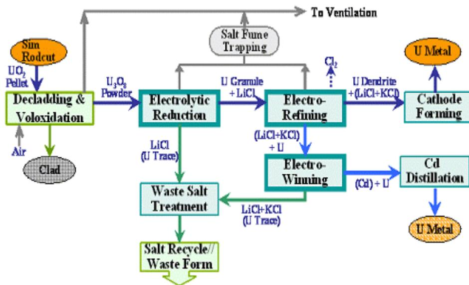
Figure 1. Process flow diagram of PRIDE
