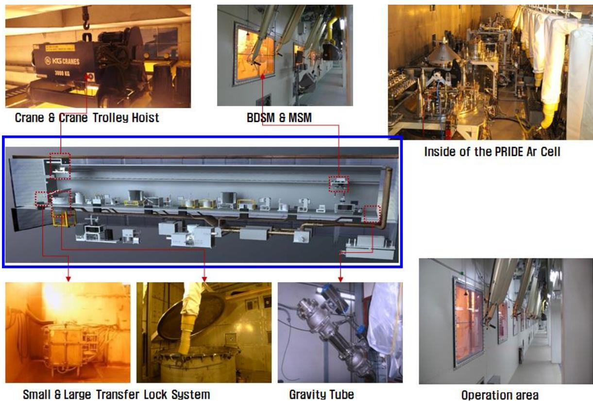
Figure 6. Operation and remote handling systems of PRIDE
