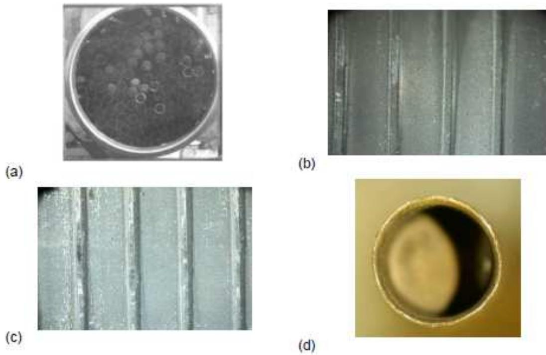
Figure 8: Visual inspection and photography of long stored pins showing (a) receipt inspection in slotted can (b) general cladding condition (c) minor handling damage on clad surface (d) end cap condition
