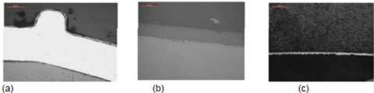
Figure 9: Metallographic examination of long stored pin cross section showing (a) clad and fuel interface as-polished (b) clad outer surface as-polished (c) etched cladding microstructure associated with RIS
