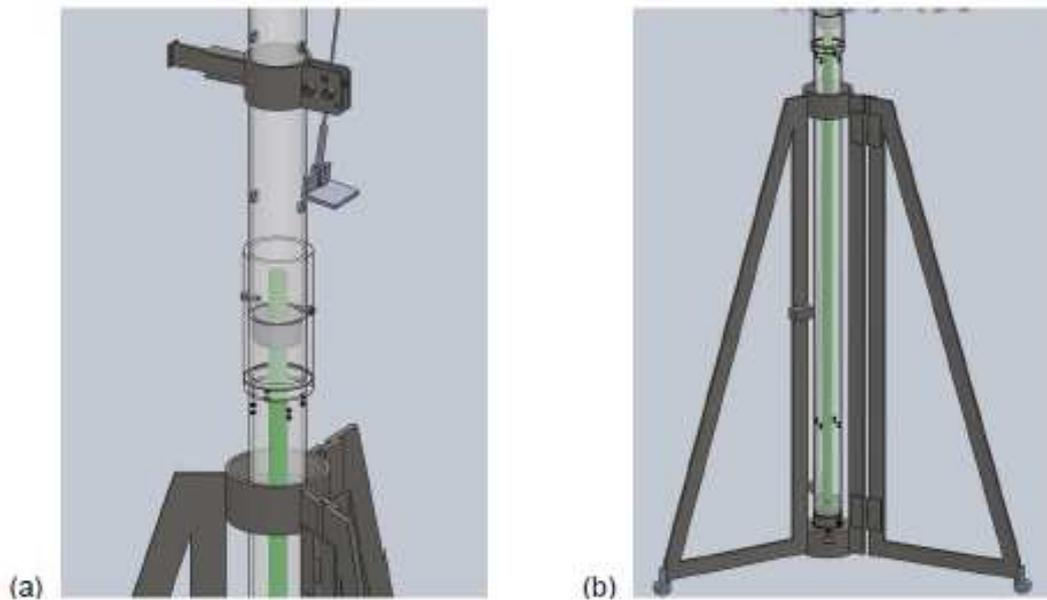
Figure 4: Impact testing rig drawing for long stored fuel (a) mid-point of assembled rig and tube holding fuel pin (b) assembled rig in vertical test position
