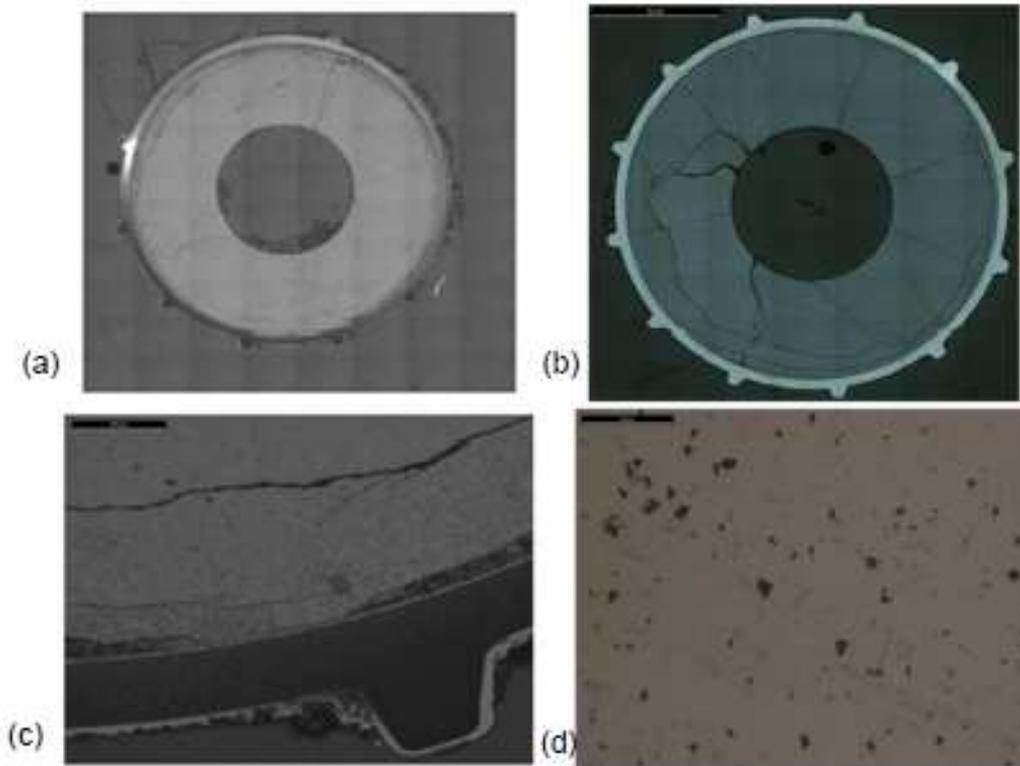
Figure 10: Metallographic images of AGR cladding microstructure from a higher burn up fuel stringer showing (a) cross section of etched fuel from a sensitised pin (b) cross section of fuel from a non-sensitised pin (c) cladding microstructure associated with RIS (d) typical clad microstructure of cladding operating at higher temperatures
