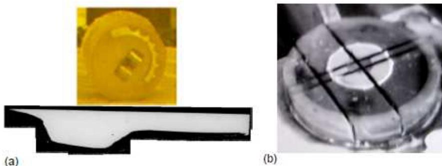
Figure 5: AGR cladding strips being prepared for electron microscopy examination (a) SEM mount and clad cross-section (b) TEM
