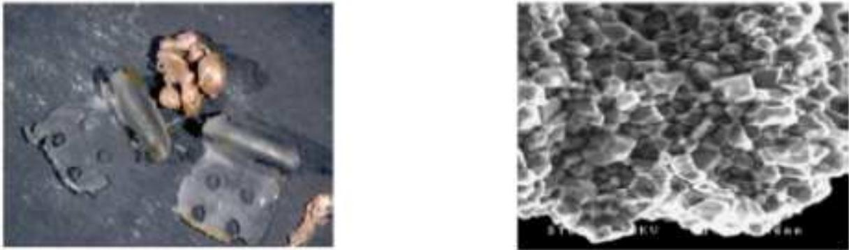
Figure 6: Irradiated AGR brace sections after strauss testing and an SEM micrograph of grain faces (SNAB) [11]
