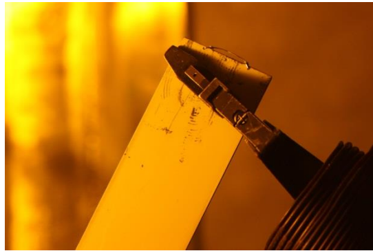
Figure 6. Wire in the top of plate fuel element
