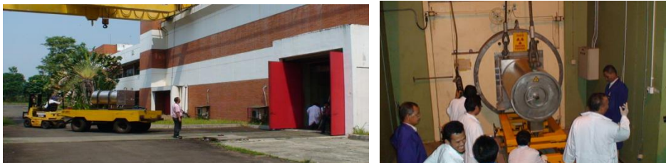
Figure 7. Process transfer of fuel plate with transfer cask.
