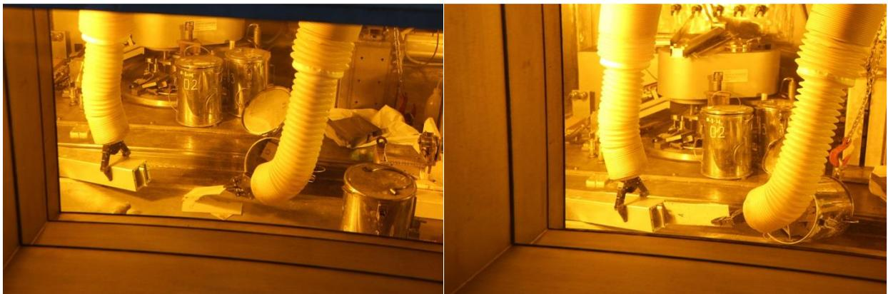
Figure 9. spent fuel plate put into containers by manipulator
