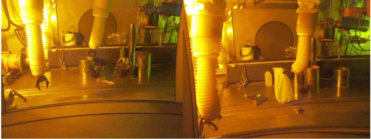
Figure 11. Hotcell 03 after mechanical decontamination (dry and wet)
