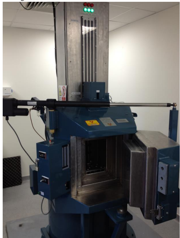
Figure 3. ^{60}\text{Co} gamma irradiator, Foss Therapy Service, Inc. [8]
