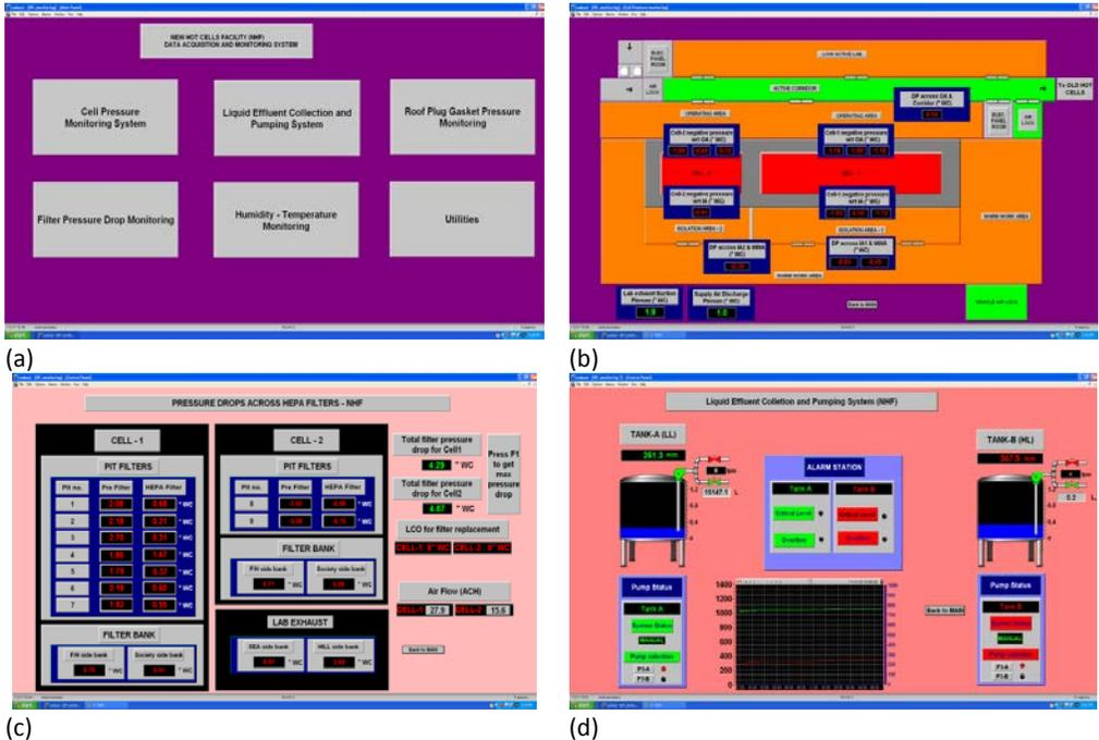
Figure. 5 (a) Centralised data acquisition and monitoring system, (b) Differential pressure monitoring of radioactive areas, (c) Pressure drop monitoring across the cell & lab exhaust filters, (d) Liquid effluent collection and pumping system monitoring console
