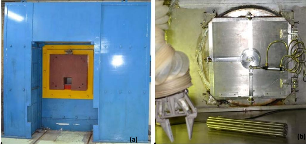
Figure 4: (a) Cold side and (b) hot side of the transfer port in the new hot cell.
