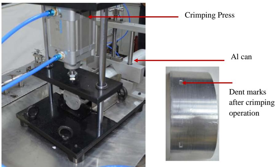
Fig.19. Crimping press assembly for the crimping the threaded end of the Aluminium cans
