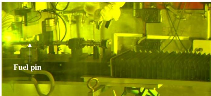
Figure 13: Scanning stage for profilometry and gamma scanning inside the hot cells.
