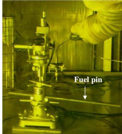
Figure 14: Puncturing set up in the hot cell for measurement of the fission gas release.
