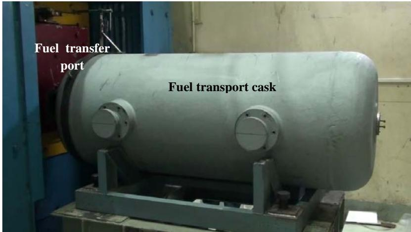
Figure 7: Docking of the fuel transport cask with the fuel transfer port of the hot cell.
