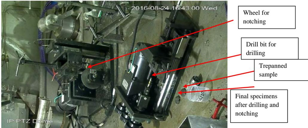
Figure 17: Drilling and notching set-up inside the cell
