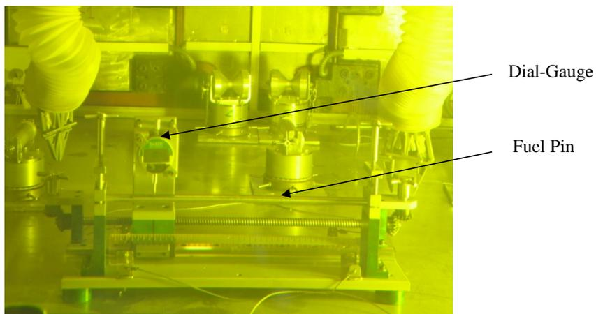
Figure 15. Bow measurement set-up
