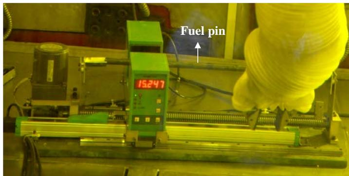
Figure 11: Laser profilometer inside the hot cell.
