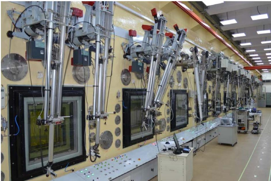
Figure 1: Operating area of the hot cells in the NHF showing the viewing windows and master slave manipulators.
