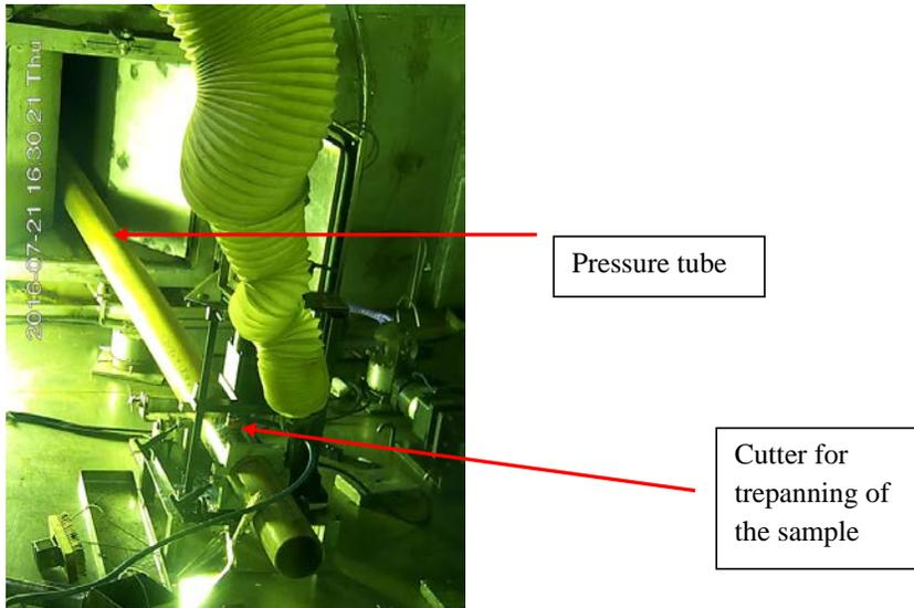
Figure 16. Trepanning of the disc compact specimens from the full length pressure tube
