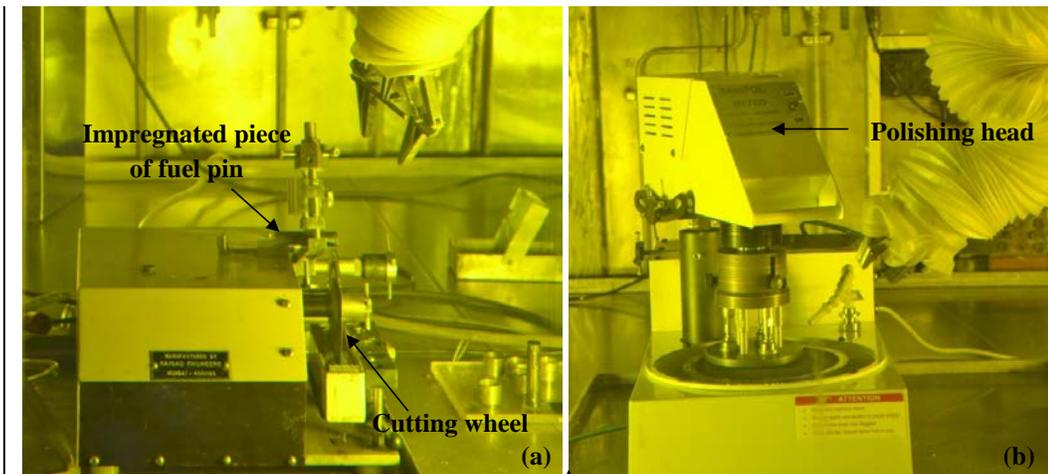
Figure 18: (a) slow speed cut off machine for cutting of metallographic samples (b) remotely operated grinder polisher inside the hot cells.
