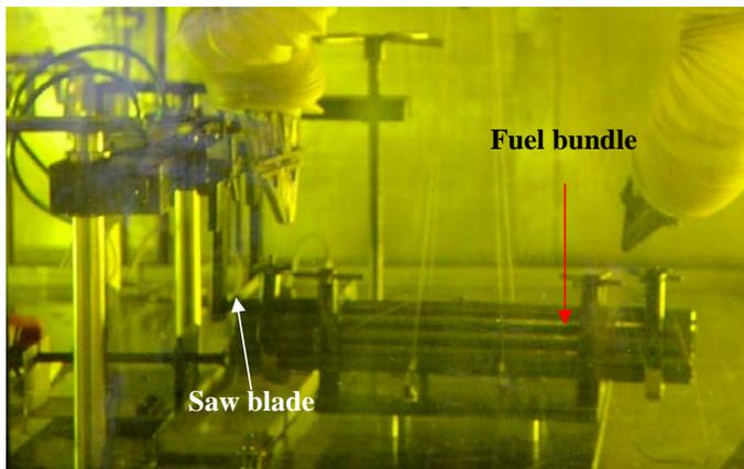
Figure 8: Saw blade based mechanical bundle dismantling machine installed inside the hot cells.
