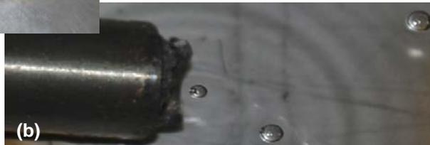
Figure 9: (a) Liquid nitrogen- alcohol leak testing set-up inside the hot cell and (b) bubbles emanating from the failure location in the fuel pin.
