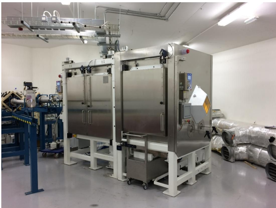
Figure 2 – Dalton End of Beamline Pelletron Accelerator Target Handling and Storage Hot Cells
