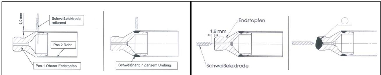
**Figure 6: Circumferential and Spot weldings**
