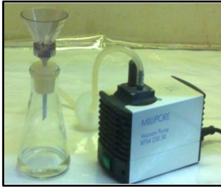
Fig. 3. Gelman filtration system equipped with vacuum pump
