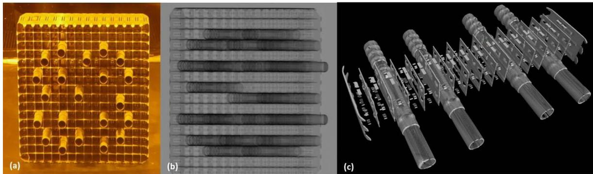
Figure 5. (a) PWR spacer grid, (b) 2D scan image and (c) a part of the spacer grid 3D scan image
