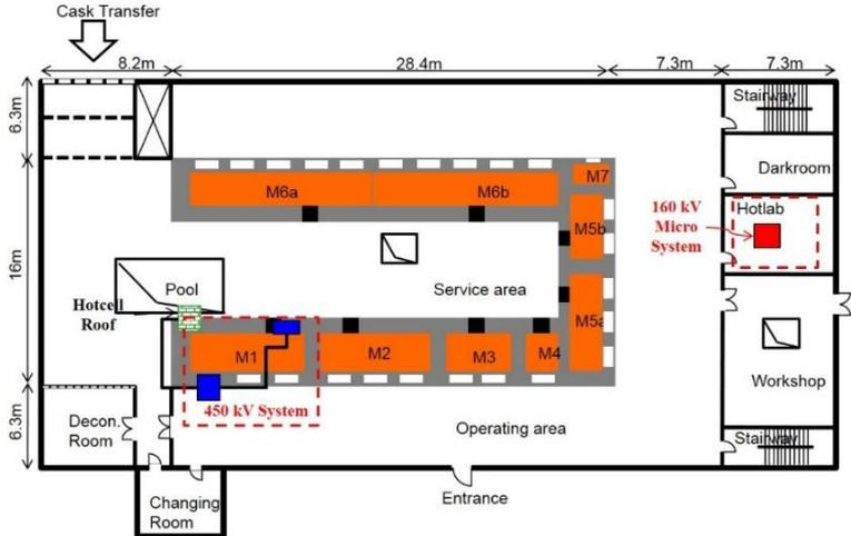
Figure 1. Installation place of the 160kV and 450kV X-ray systems
