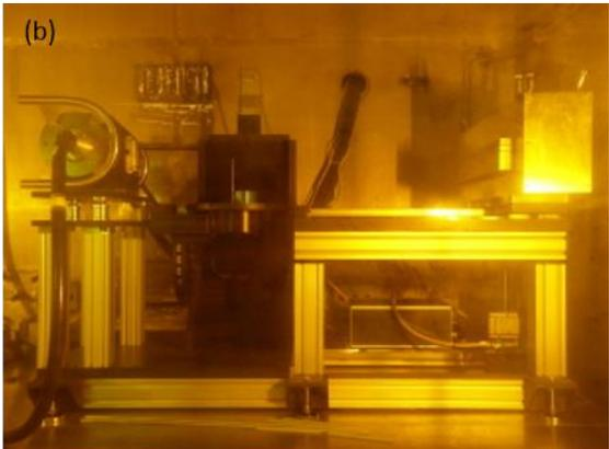
Figure 2. 450kV X-ray system (a) layout and (b) installation in hotcell
