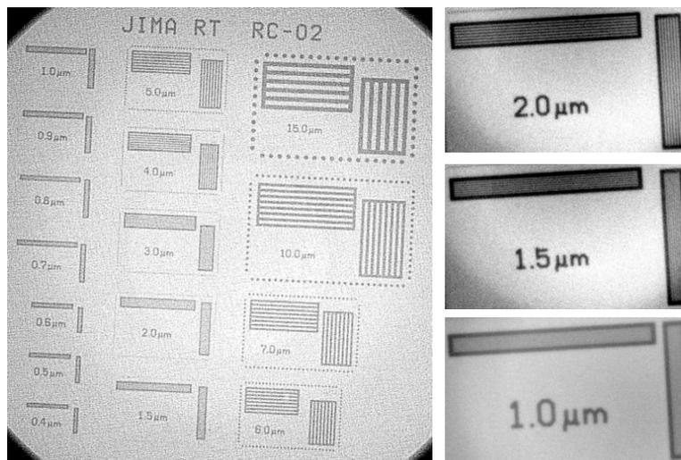
Figure 7. Resolution measuring result of 160kV X-ray
