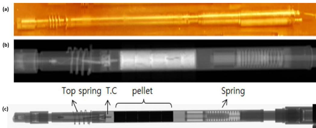
Figure 4. (a)  $\text{UO}_2$  fuel rod (b) 3-D scan image (c) 2-D scan image
