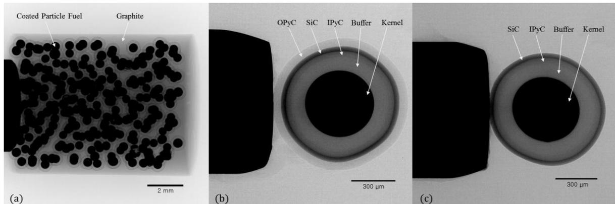
Figure 8. X-ray image of (a) Un-irradiated fuel compact, (b) Un-irradiated coated particle fuel, and (c) irradiated coated particle fuel
