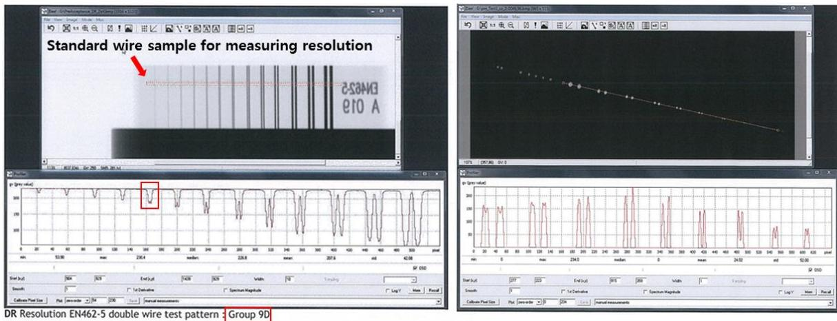
Figure 3. Resolution measuring results of the 450kV X-ray system (Group 9D: 0.130 mm)
