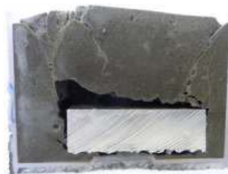
Fig. 3: Consequences of corrosion by cementation on aluminum massive bloc
