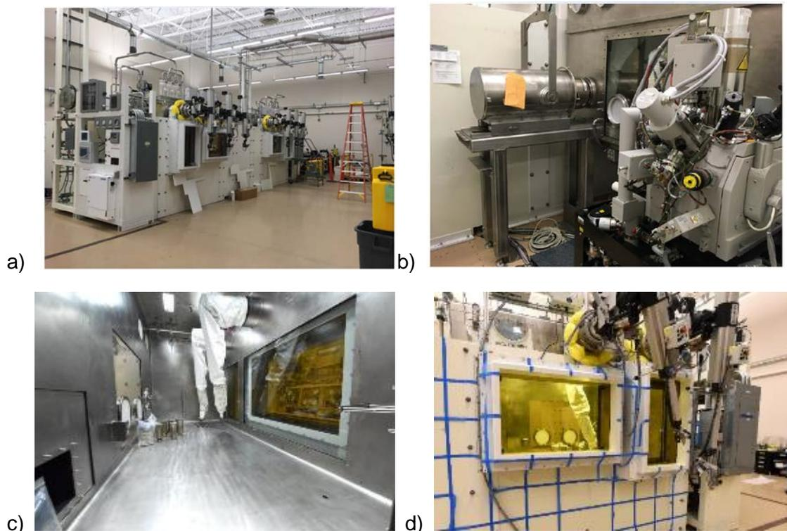
Figure 5: a) Manipulator workstations of the FIB's SAS cell, b) image of the inside of the Quanta FIB SAS showing the instrument and the transfer cask, and c) image of inside of one of the FIB SAS gloveboxes, and d) image of the manipulator workstation.
