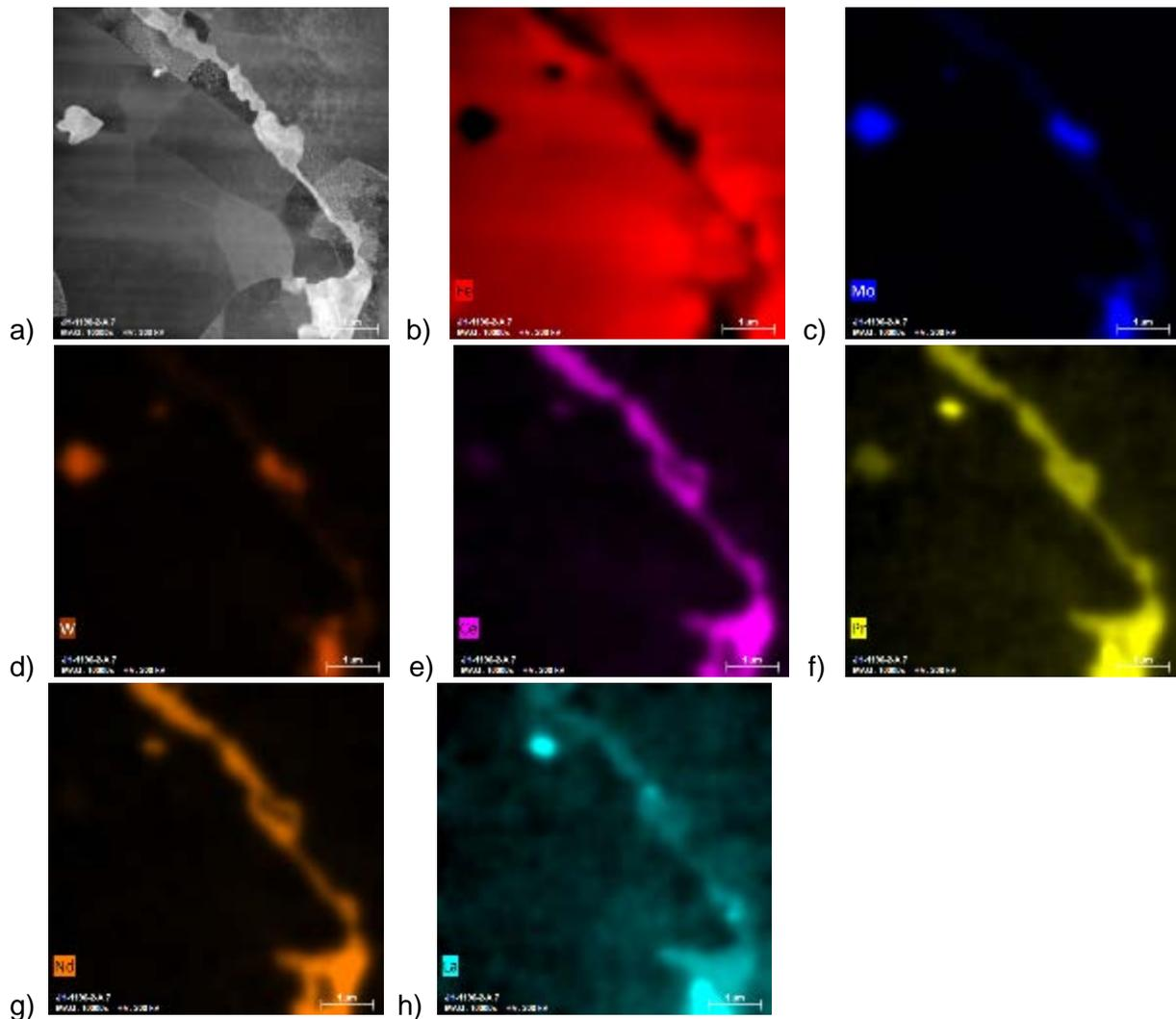
Figure 12: EDS maps of rare earth elements diffusing into HT-9 cladding. a) HAADF, b) Fe, c) Mo, d) W, e) Ce, f) Pr, g) Nd, and h) La. Scale bar is 1  $\mu\text{m}$ .
