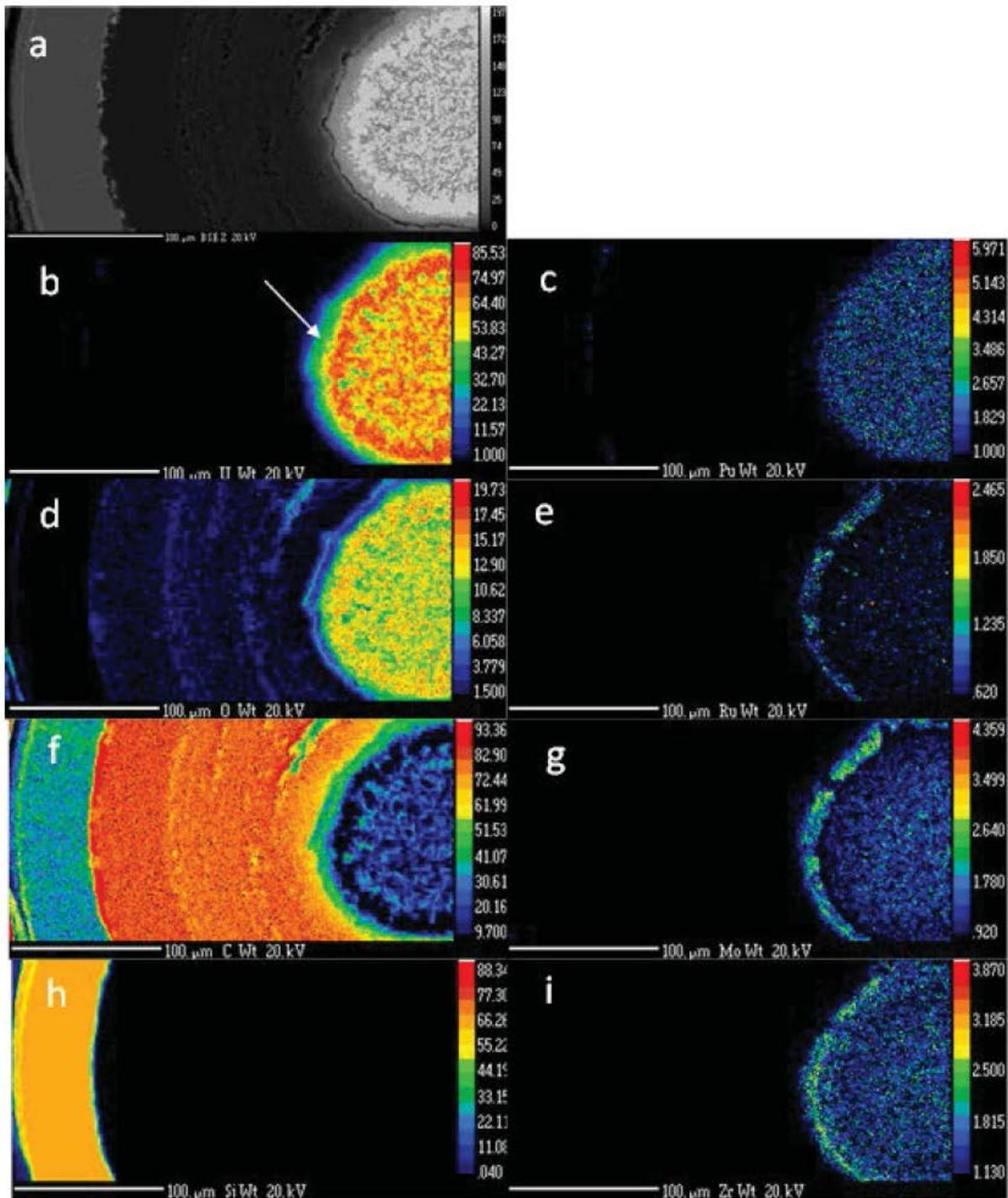
Figure 13: EPMA measurements of an irradiated TRISO fuel particle: a) SEM micrograph, b) U, c) Pu, d) O, e) Ru, f) C, g) Mo, h) Si, and i) Zr (1).
