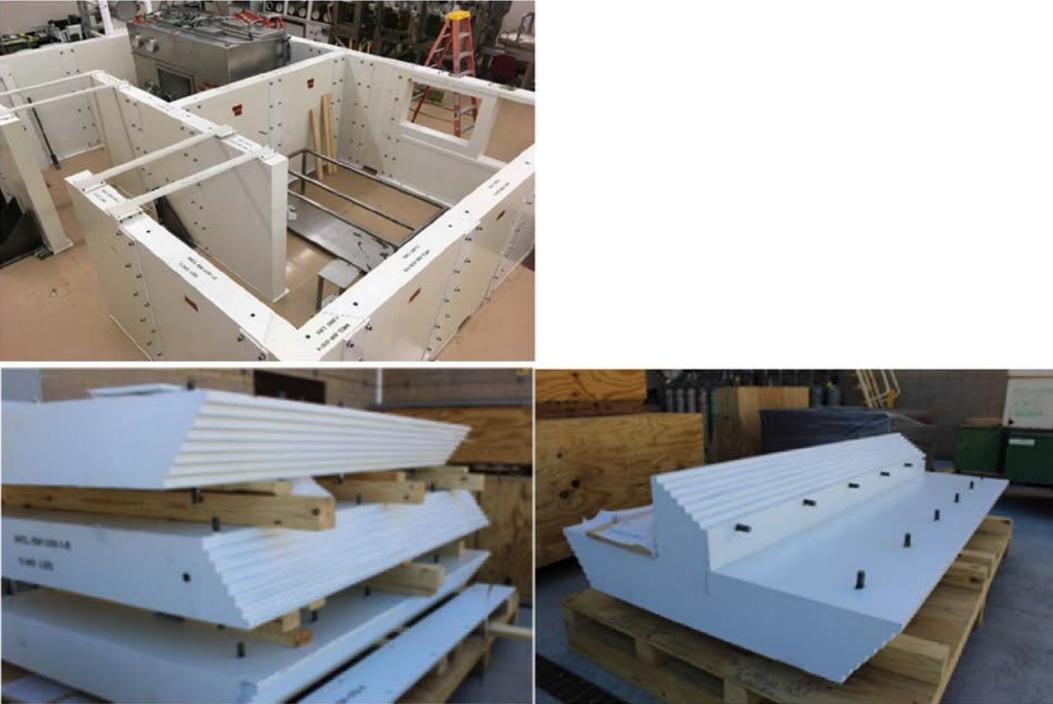
Figure 2: FIB/PFIB SAS layout and various steel sections that compose the shielding
