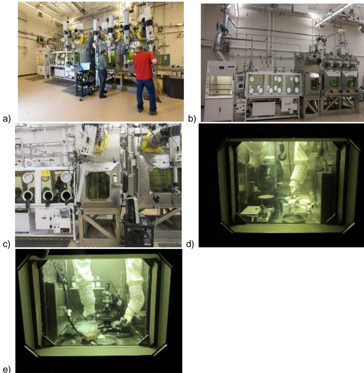
Figure 4: Images of the SSPA showing a) and b) the overall SSPA line, c) the sample transfer cell, d) the sample preparation bay, and e) the optical microscopy bay.
