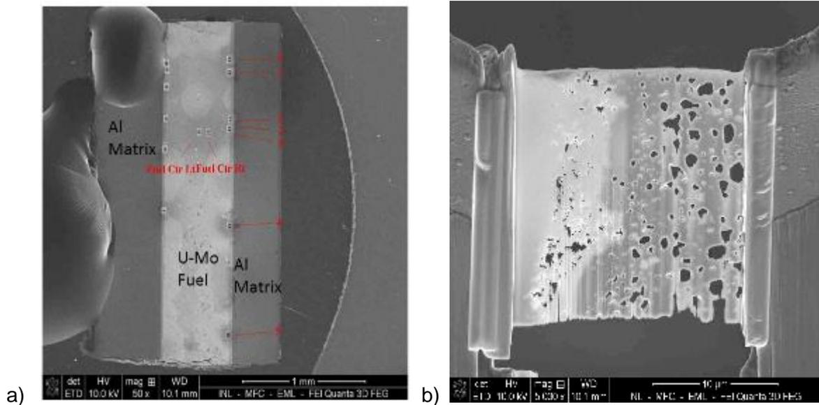
Figure 9: FIB micrographs showing the irradiated microstructure of irradiated U-Mo fuel during TEM sample preparation. Serial sectioning using the FIB on cubes provides useful information on the morphology of defects/microstructure of a material.
