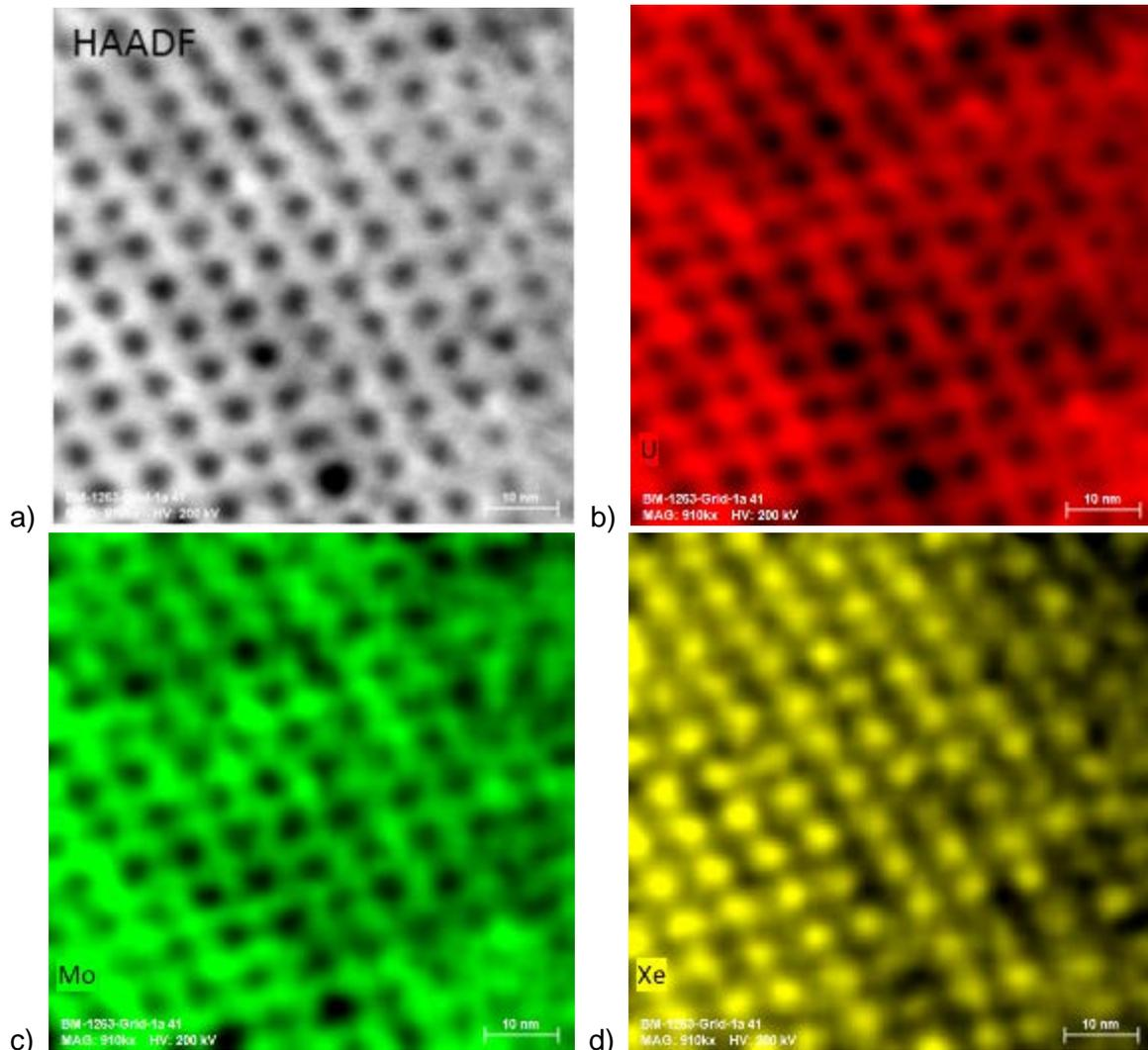
Figure 11: EDS maps of irradiated U-Mo fuels showing the a) HAADF micrograph, b) U, c) Mo, and d) Xe.
