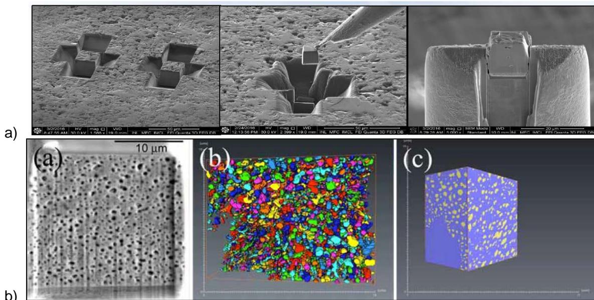
Figure 10: FIB micrographs showing cube/serial sectioning work on irradiated  $UO_2$  and U-Mo fuel. a) cube preparation of  $UO_2$ , b) micrographs showing the serial section of U-Mo and its porosity reconstructions.
