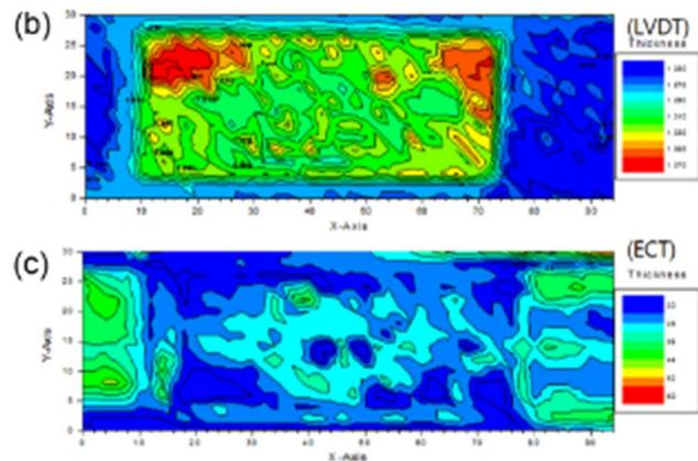
Figure 7. (a) 2-D dimensional measurement for plate fuel, (b) example of thickness measurement, and (c) example of oxide thickness measurement
