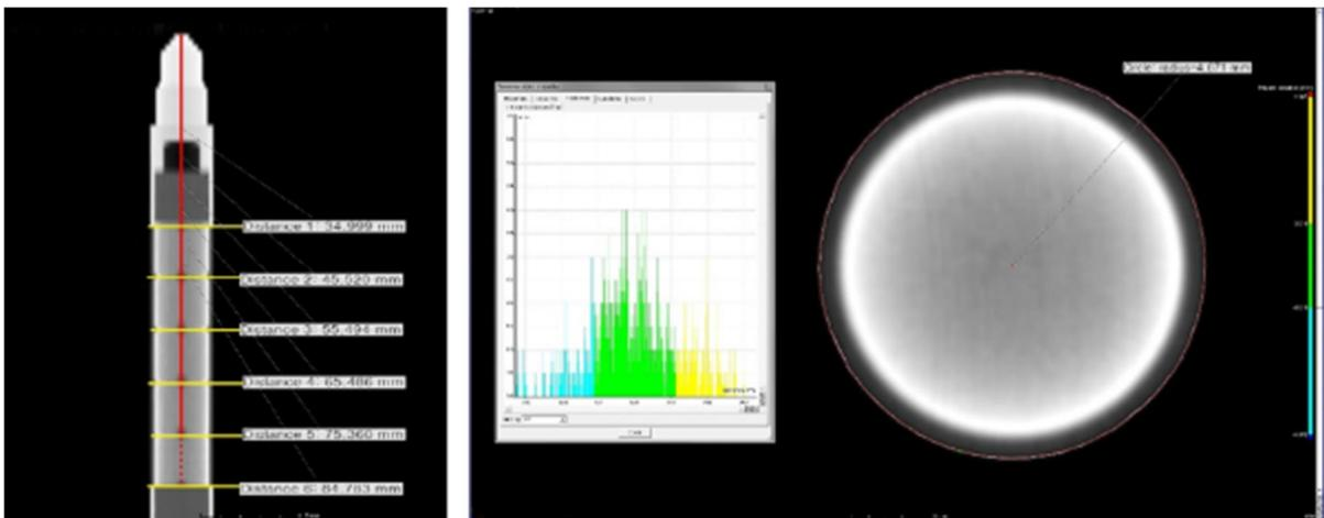
Figure 5. Dimensional measurement of R&D fuel
