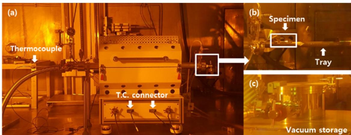
Figure 10. Vacuum heating system installed in hotcell
