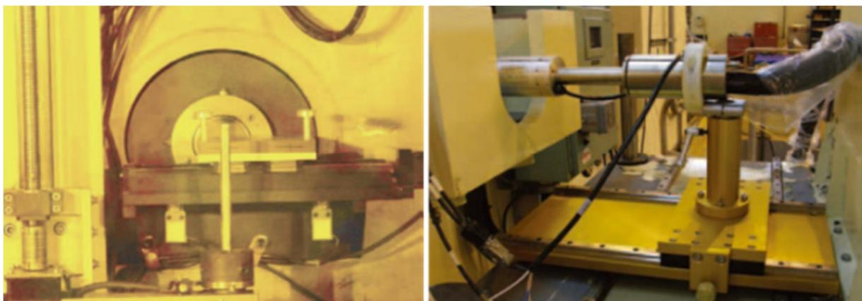
Figure 8. Gamma scanning system and HPGe detector
