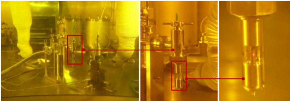
Figure 9. Laser puncturing system installed in hotcell
