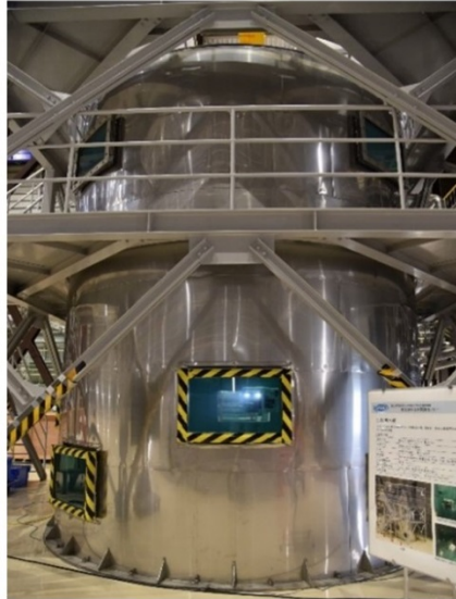
Fig. 5 Robot testing pool. The water diameter and the depth are 4.5 m and 5 m, respectively.
