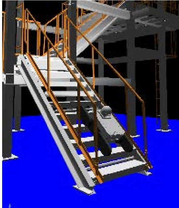
Fig. 9 Screen grab from the display of the robot simulator. A robot is working at the mock-up stairs for preparation of the decommissioning.
