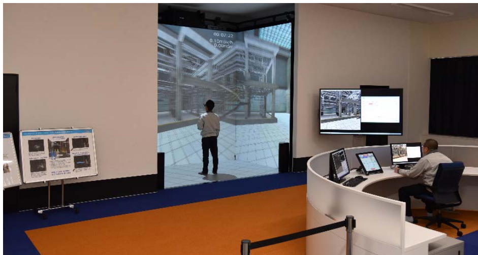
Fig. 7 Cave type 4-sided screen virtual reality system is installed mainly for the decommissioning of the Fukushima Daiichi Nuclear Power Station, unit 1 to unit 3. A stereographical movie is realized with 5 computers which make successive images on the 4 sided screens for each eye belong to an operator with special goggles. Various applications other than the decommissioning are also available.
