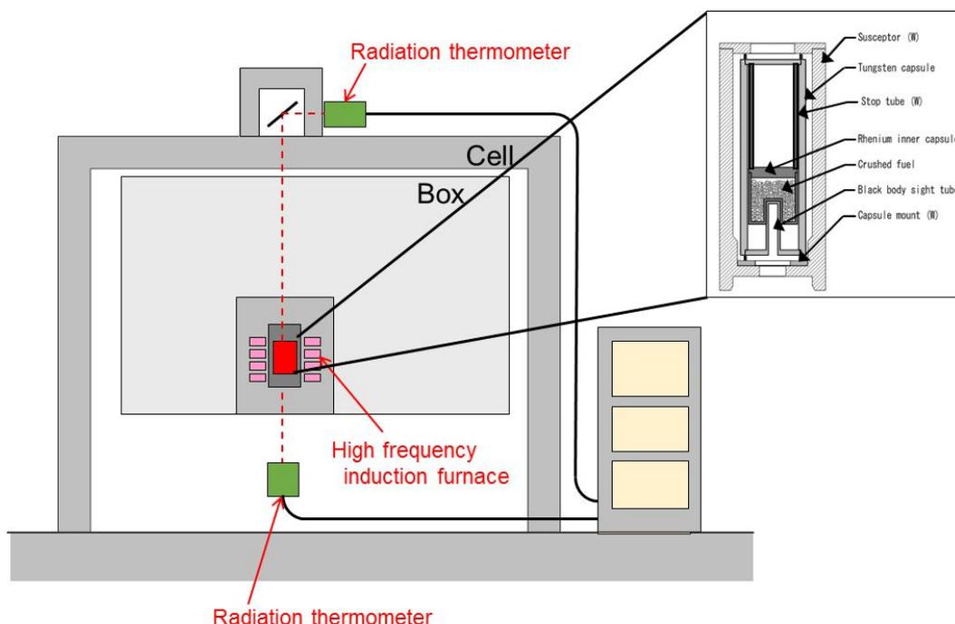
Fig. 1 Schematic illustration of the apparatus for measuring the melting temperature of irradiated fuels
