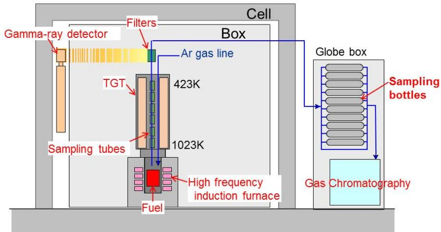
Fig. 3 Schematic illustration of the FP release behavior test apparatus
