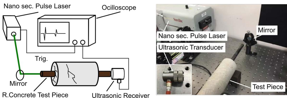
Fig.4 Schematic illustration of experimental method (Left) and the actual system (Right).
