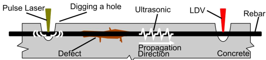
Fig.2: Concept of the remote testing method for reinforced concrete structure
