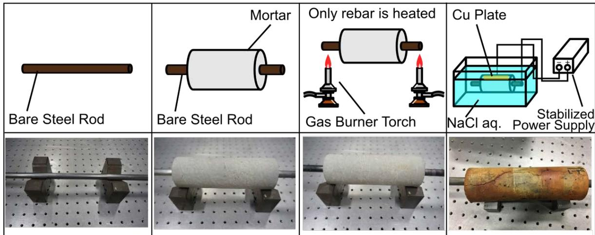
Fig.3 Schematic illustrations of each test piece and the actual photos: (a) bare steel rod, (b) sound reinforced concrete, (c) heated reinforced concrete and (d) electrically corroded reinforced concrete, respectively.
