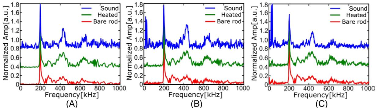
Fig.6 Normalized frequency spectrum of the ultrasonic signals: (A) is corresponding to the Fig.5 (a) signals, (B) is Fig.5(b) and (C) is Fig.5 (c), respectively. Blue, green and red solid lines represent sound test piece, heated test piece and bare rod, respectively.
