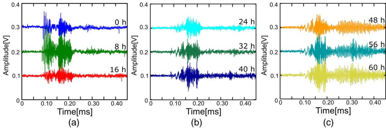
Fig.7 Ultrasonic waveforms of the corroded test piece with each 8 hours energization time. (a) is from 0 hour to 16 hours, (b) is from 24 hours to 40 hours and (c) is from 48 hours to 60 hours.
