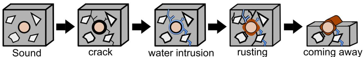
Fig.1: The deterioration process of reinforced concrete
