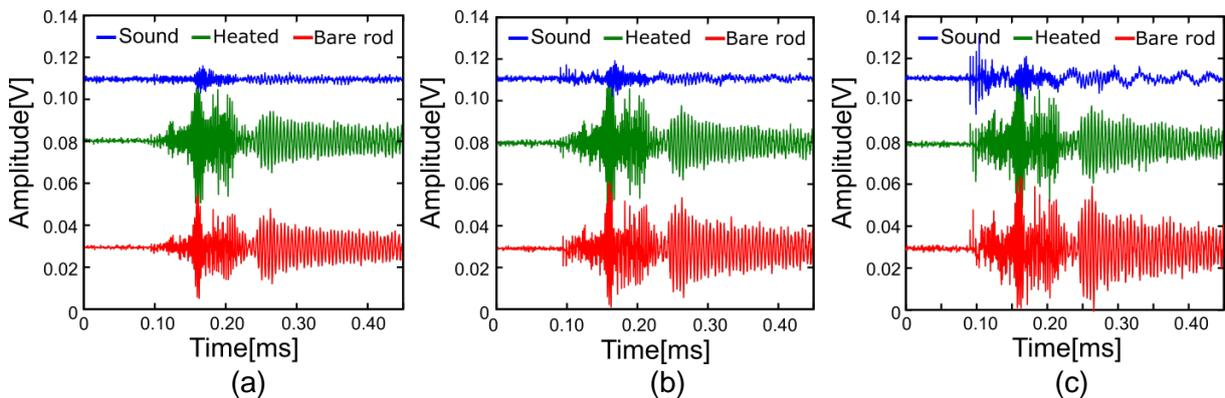
Fig.5 Ultrasonic waveforms: (a) is 60 mJ of laser irradiation power, (b) is 100 mJ and (c) is 140 mJ, respectively. Blue, green and red solid lines represent sound test piece, heated test piece and bare rod, respectively.
