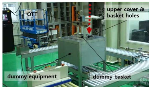
Figure 7. the holding operation
