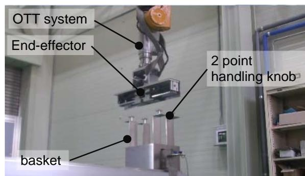
Figure 6. The integrated OTT system and its end effector for basket handling.
