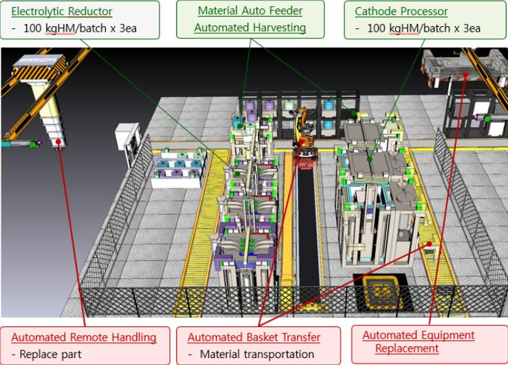
Figure 1. The virtual 3D simulation for evaluation of automation concept [6].
