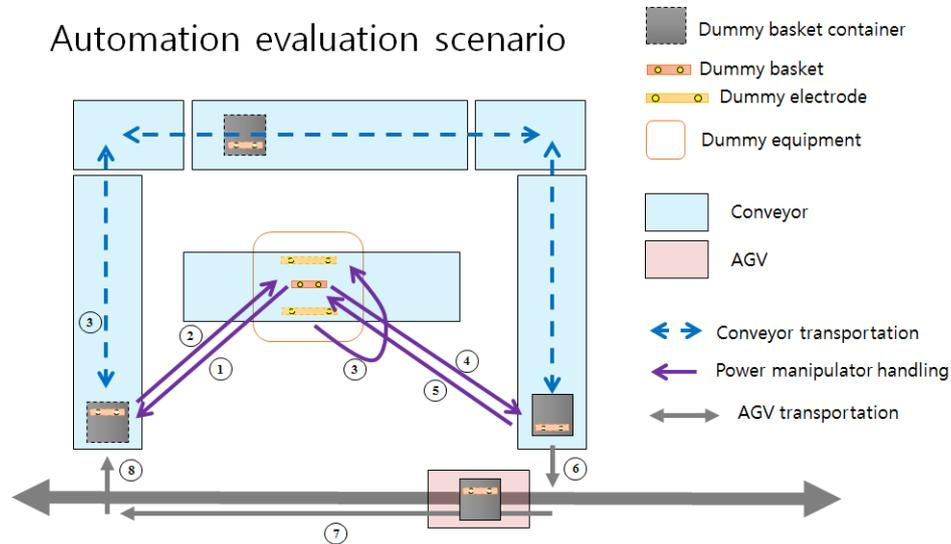
Figure 3. Evaluation scenario for pyroprocessing automation concept.
