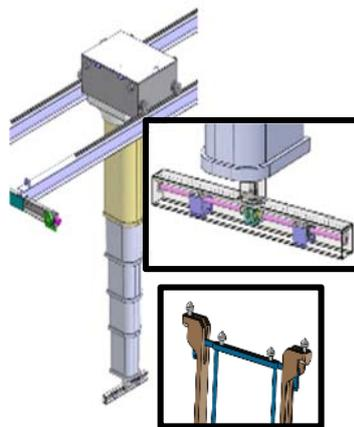
Figure 4. The proposed OTT system with T-shaped gripper for basket handling
