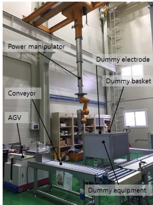
Figure 5. The integrated automation testbed
