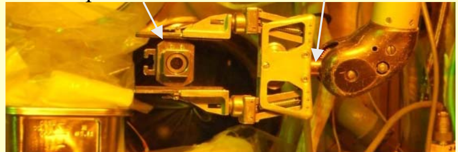
Photo of the specimen holder in the shielded hot cell
