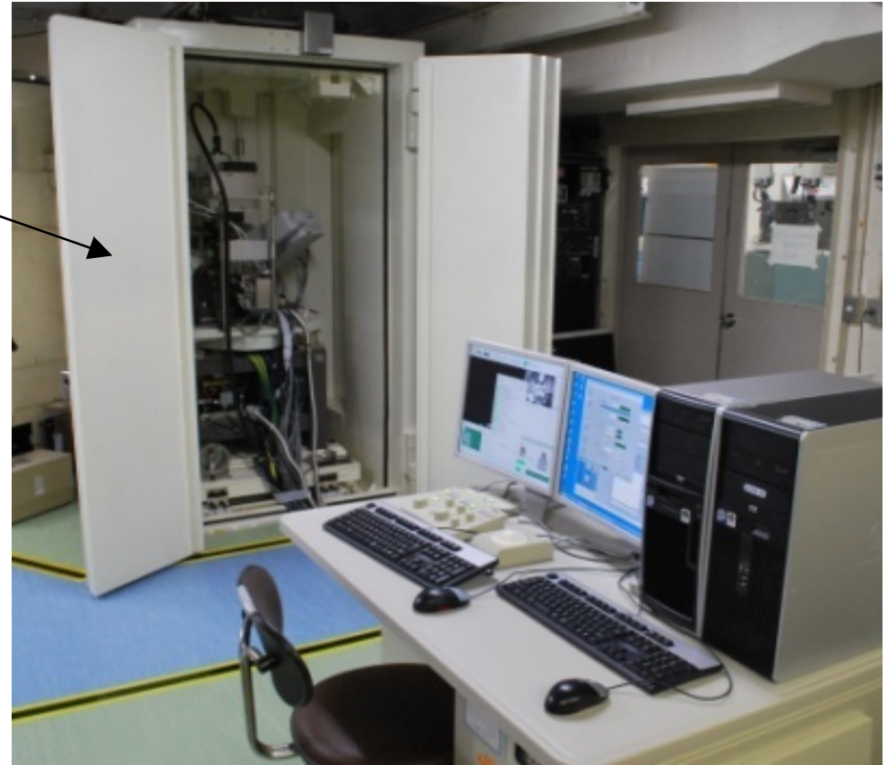
Photo of the modified FE-SEM and lead shield box.
