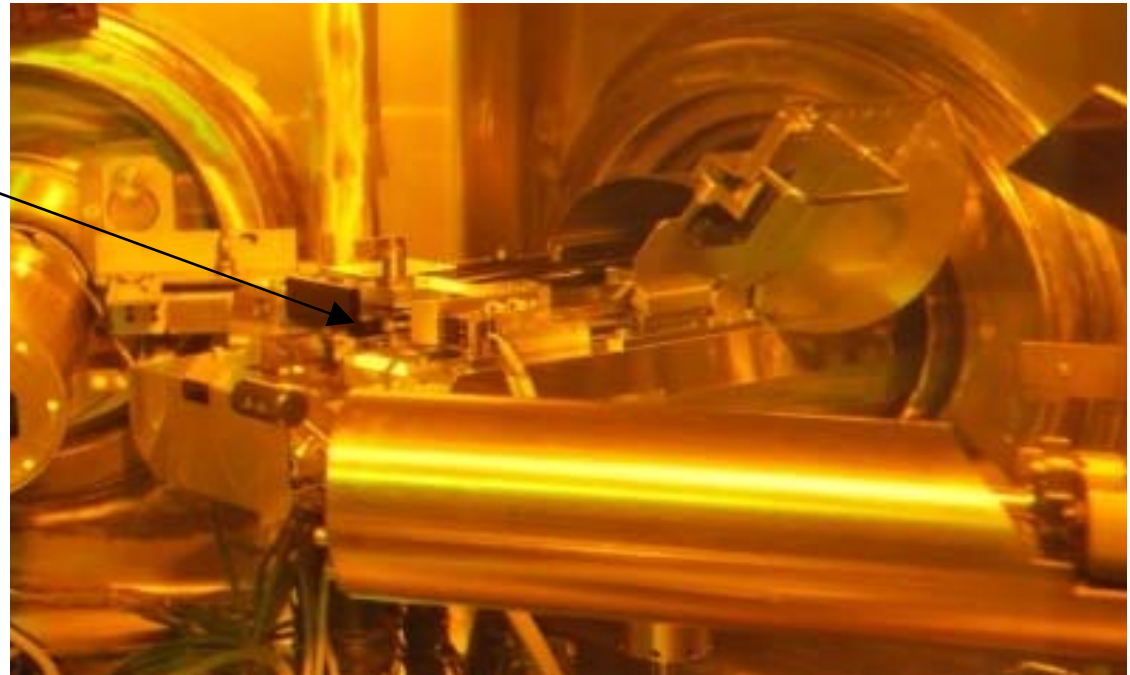
Photo of the specimen transfer unit in the shielded hot cell.
