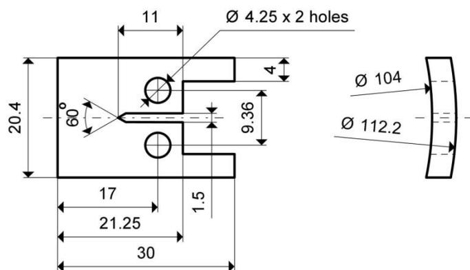
Figure 54: CT sample ASTM 399
