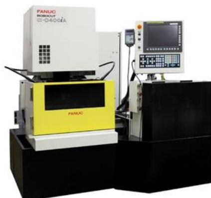
Figure P9: The FANUC ROBOCUT α-C400iA has controls (right) separated from the EDM system (left).
