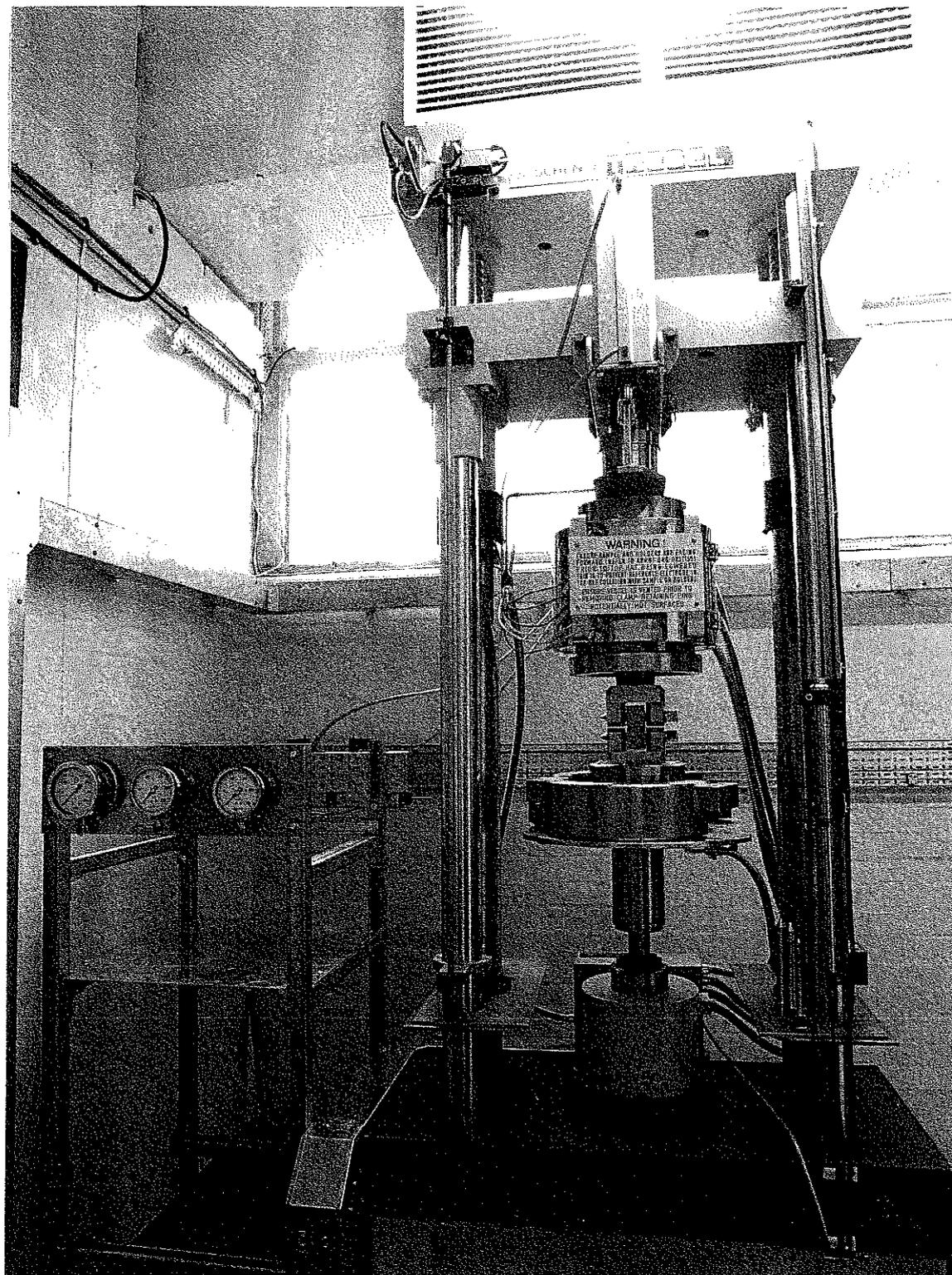
Fig 2: 100KN Testing Machine fitted with autoclave and clevises for CTS specimens.
