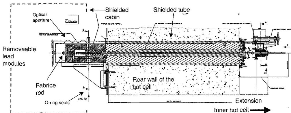
**Figure 4** Layout of the fuel rod positioner
