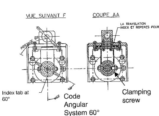
Figure 7 : Front Layout of the fuel rod positioner
