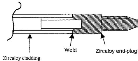
Figure 2 Weld Zircaloy end-plug
