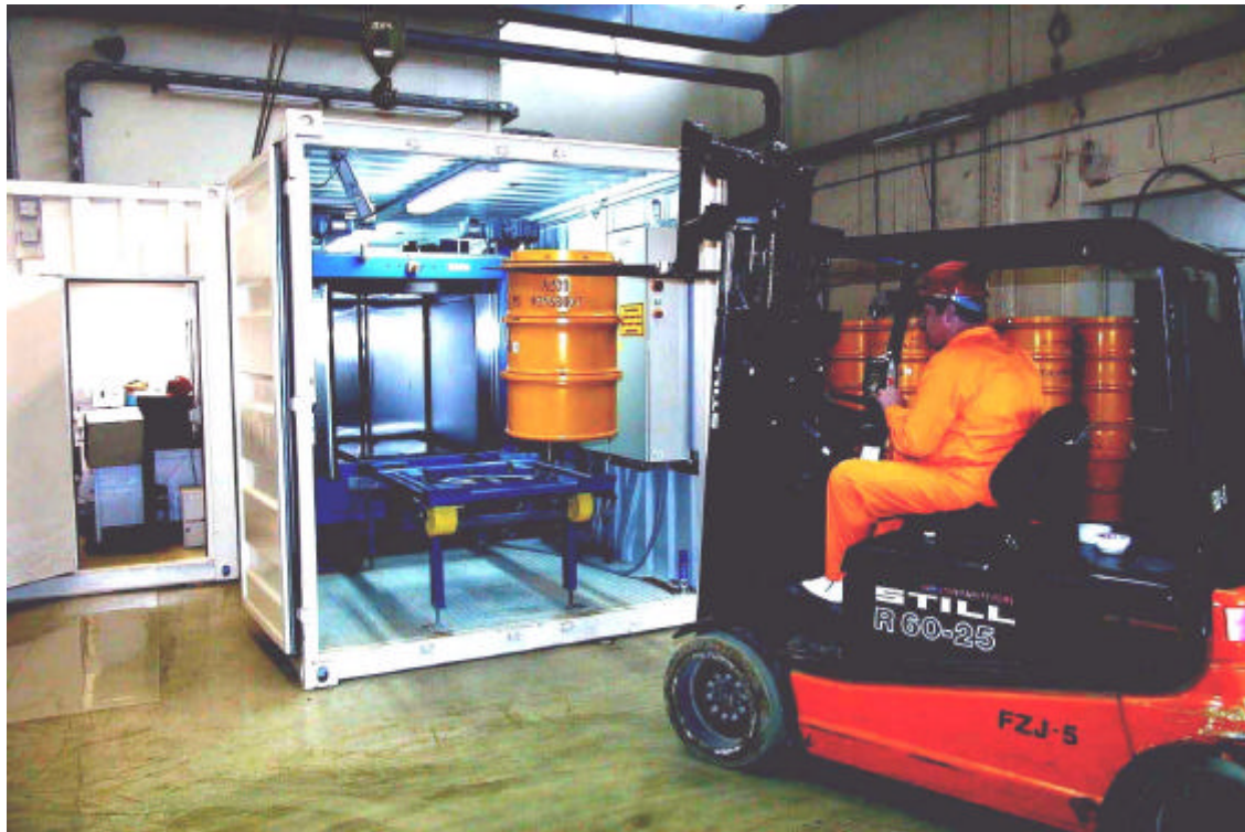
Fig.4 Clearance measurement device constructed by RADOS GmbH
