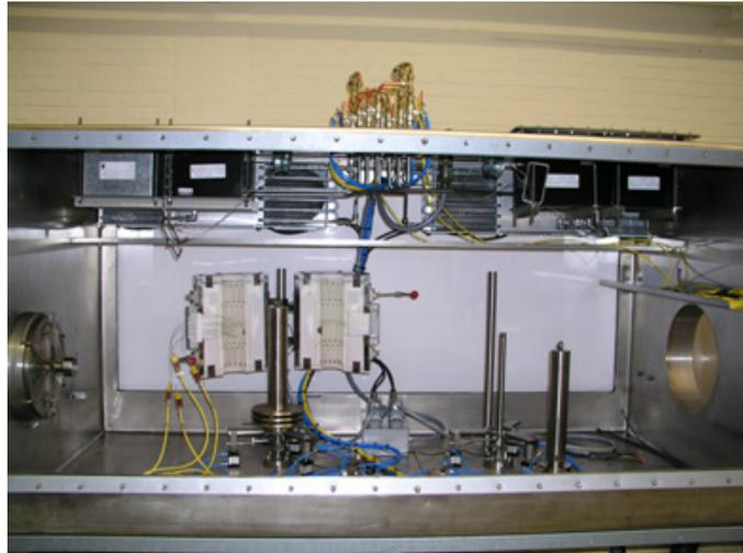
**Fig. 6** Picture of the creep test system inside a glove box
