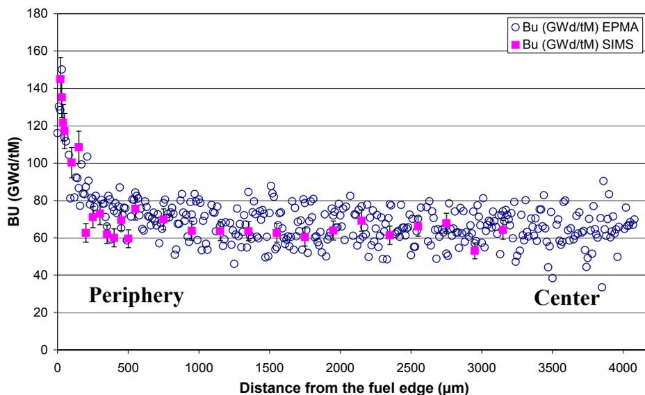
**Figure 3.** Radial burnup distribution collected on the HBU sample using SIMS and EPMA method
