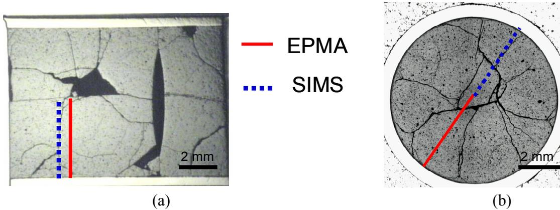
**Figure 1.** Location of EPMA and SIMS measurements on (a) LBU and (b) HBU fuel pellet
