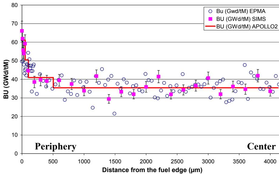
**Figure 2.** Radial burnup distribution collected on the LBU sample using SIMS and EPMA method
