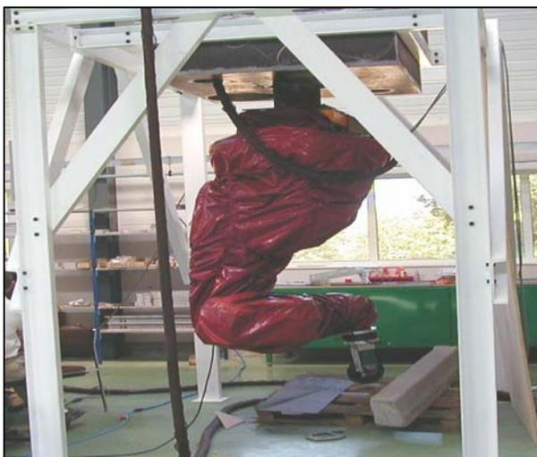
Fig. 2: RX arm equipped with booting
