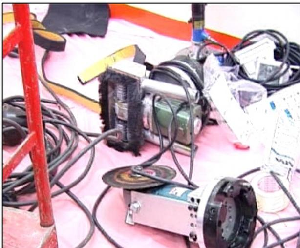
**Fig. 4:** Various tools – disk cutter and concrete scraper
