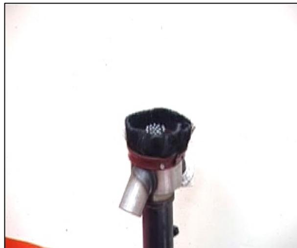
**Fig. 5:** needle scaler for concrete scabbling
