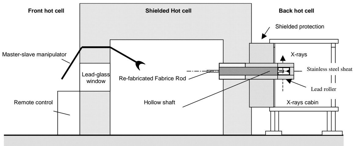
Fig.12 : radioscopy hot cell
