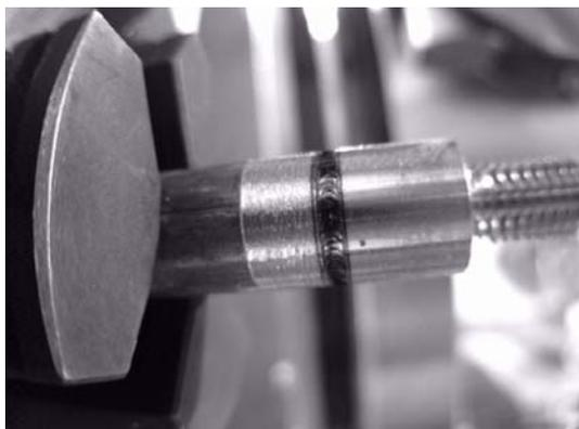
**Fig.2 : Laser welding**
