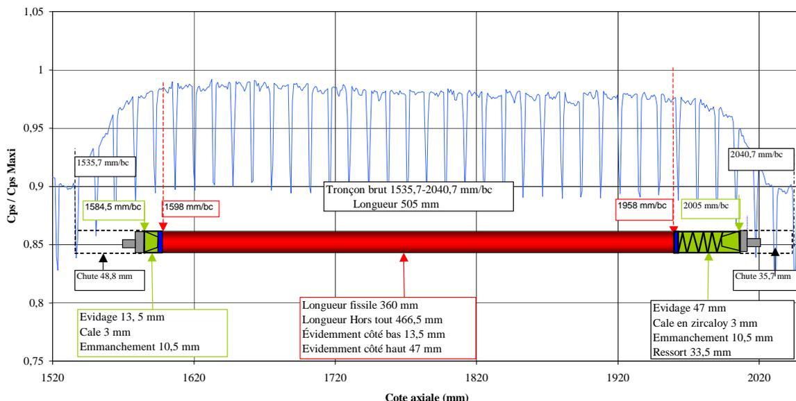
**Figure 6 :** gamma-scanning profile fuel rod
