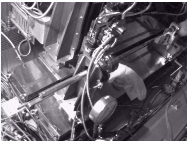
**Fig.8 :** Instrumented fuel rod
