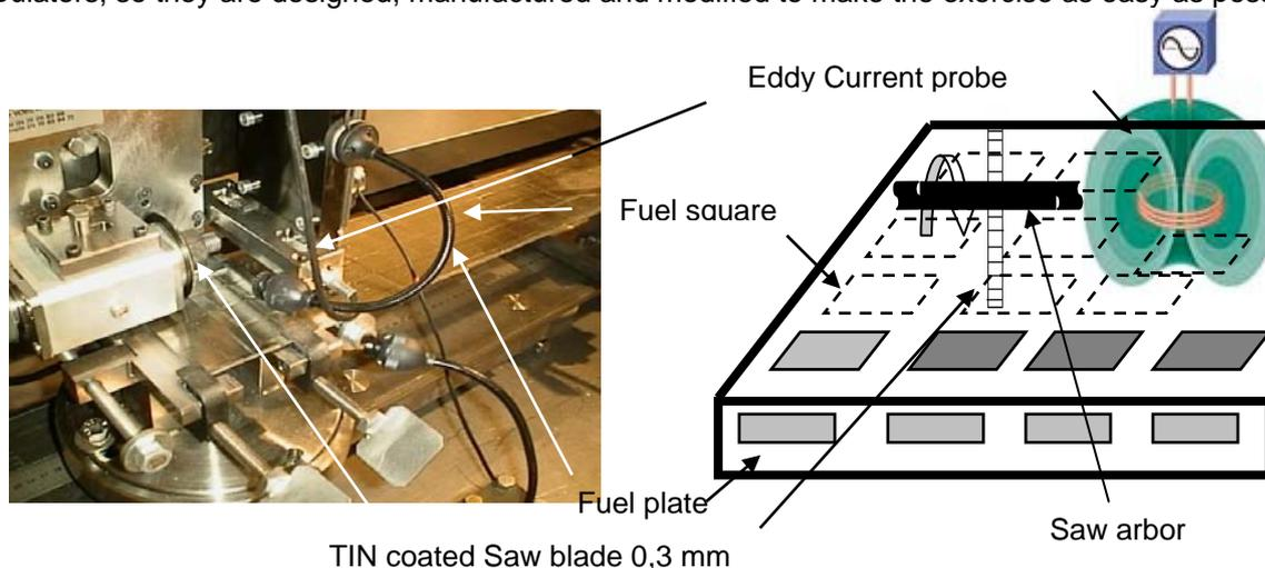
**Fig.11** : Fuel plate location by Eddy current probe
