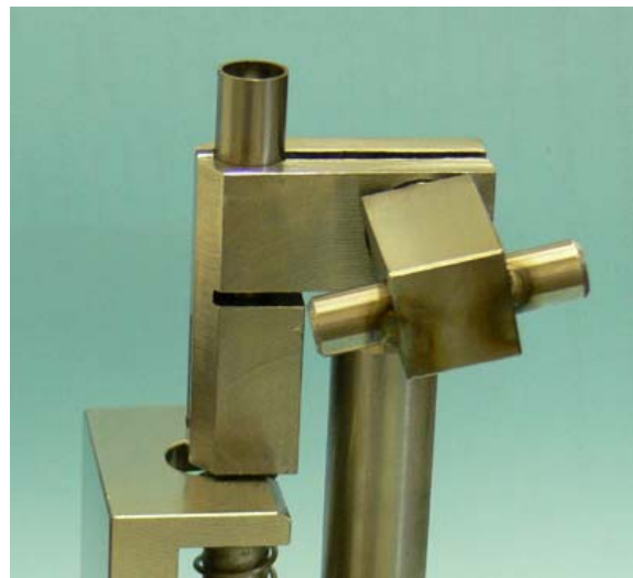
fig.8 Placing the half cylinders into the specimen
