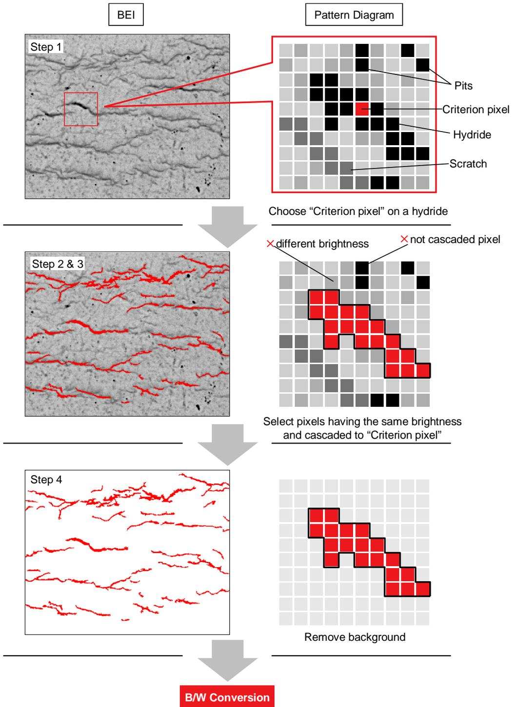
Figure 1 Schematic drawing of Color Gamut Selection Method
