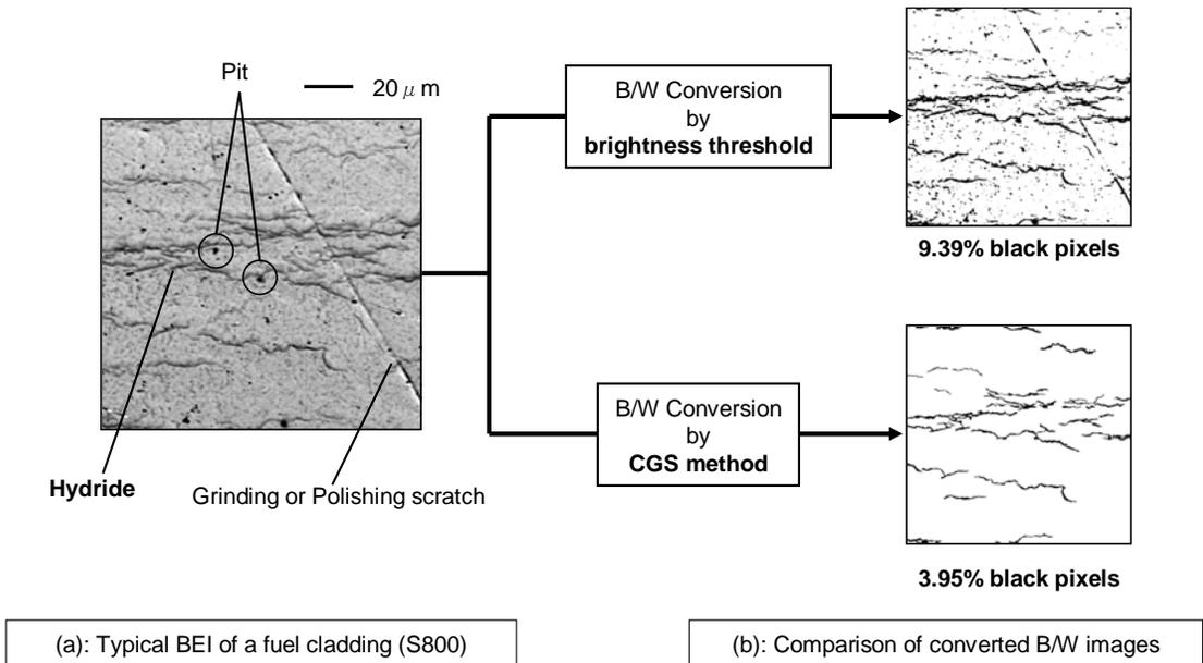
Figure 2 Typical BEI and B/W converted images
