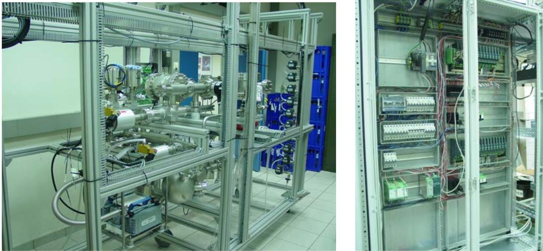
**Fig 2: Vacuum system installed on the new frame (left) – New control cabinet (right)**
