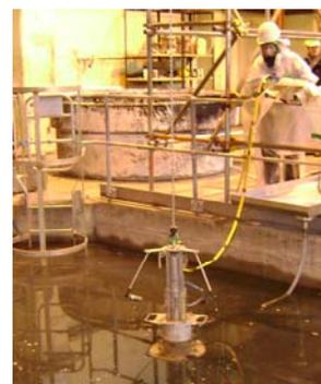
Figure 6: Bell Jar deployed in the 6m deep pit.
