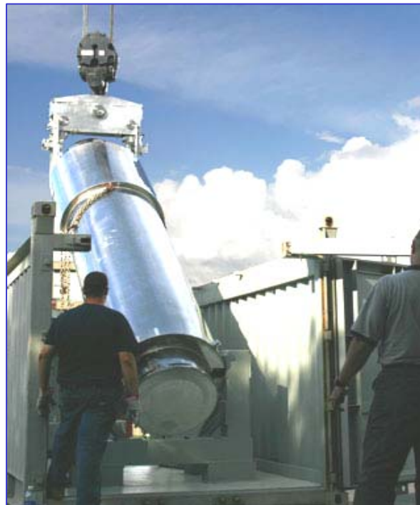
Figure II – NAC-LWT Cask being placed into its ISO container
