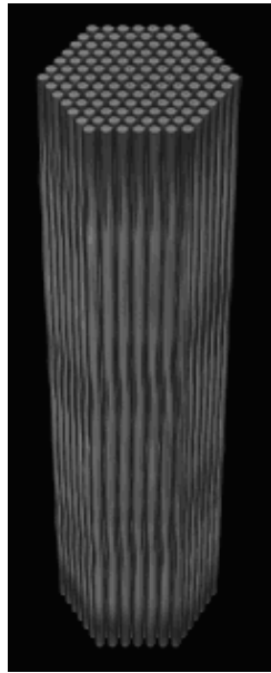
Fig.5(b) Three-dimensional X-ray CT image without duct tube
