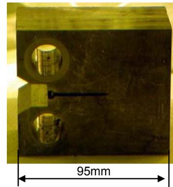
Fig.5 1.5T-CT specimen (maximum size)
