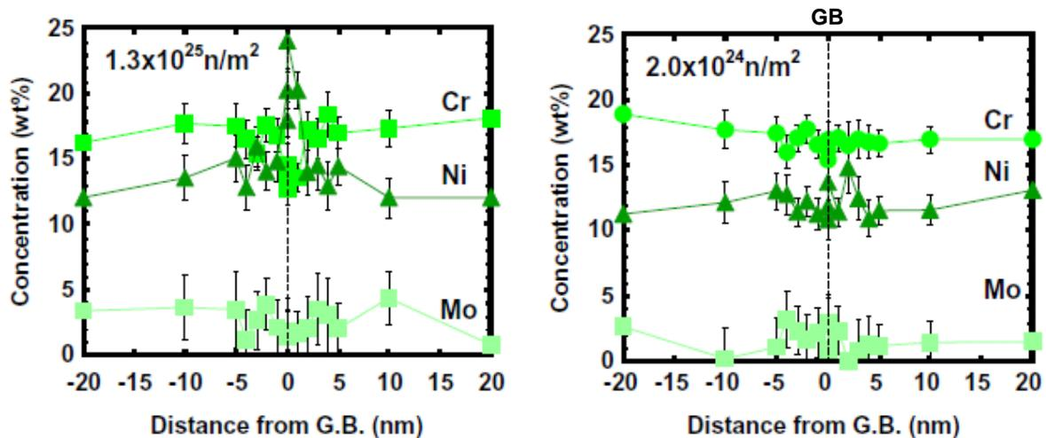
Fig.6 Example compositional profiles across a GB in irradiated Type 316 SS [10]
