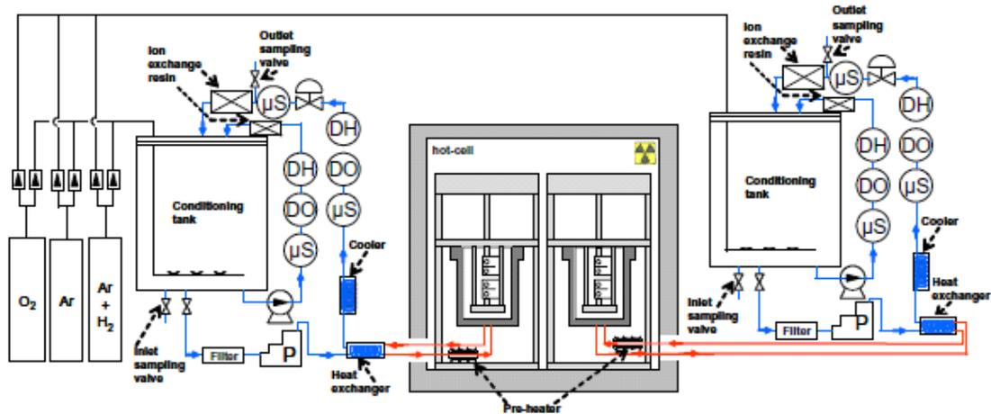
Fig.1 Schematic of CGR test facility [9]
