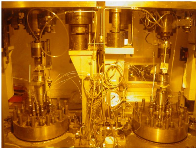
Fig.2 Photo of the equipment for the CGR test
