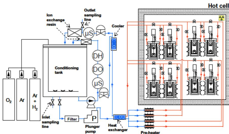
Fig.4 Schematic of SSRT/UCL test facility [10]
