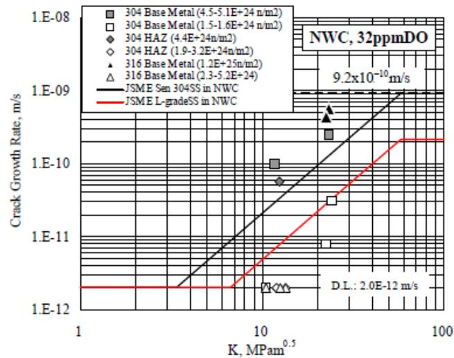
Fig.3 Dependence of CGR on neutron fluence [9]
